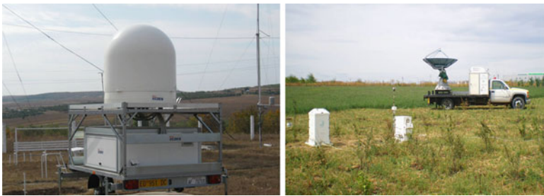
Fig. 2 A mini-radar (left) and the XPol mobile radar with disdrometer and gauges (right)
