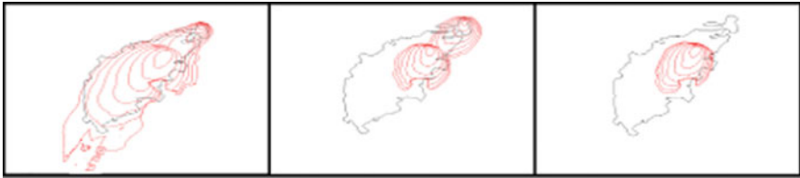
Fig. 4 Simulation of FARSITE for the fire in Voutsas on 28-07-2005 for the test 1, 2 and 3 of fuel models. The black line is the real burnt land whereas the red line shows the simulated burnt land of the fire per hour
