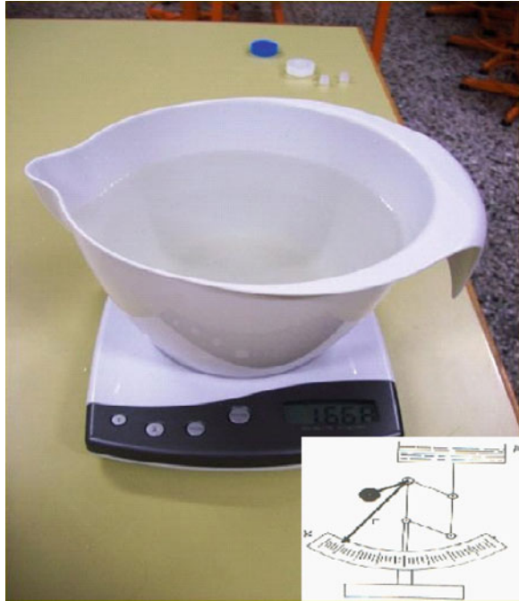
Fig. 4 The reproduction of an evaporation meter (Model instrument at lower right )
