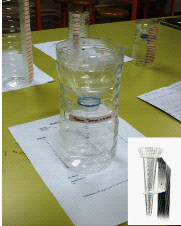
Fig. 3 The reproduction of a rain gage (Model instrument at lower right)
