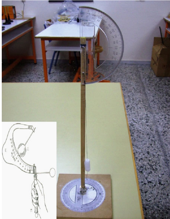
Fig. 5 The reproduction of a “Daloz” anemometer (Model instrument at lower left )
