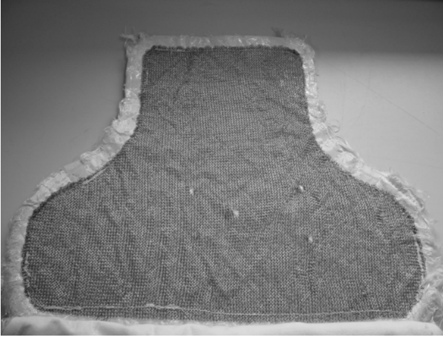
FIGURE 4-9. A representative knife armor—chain mail backed with aramid.
