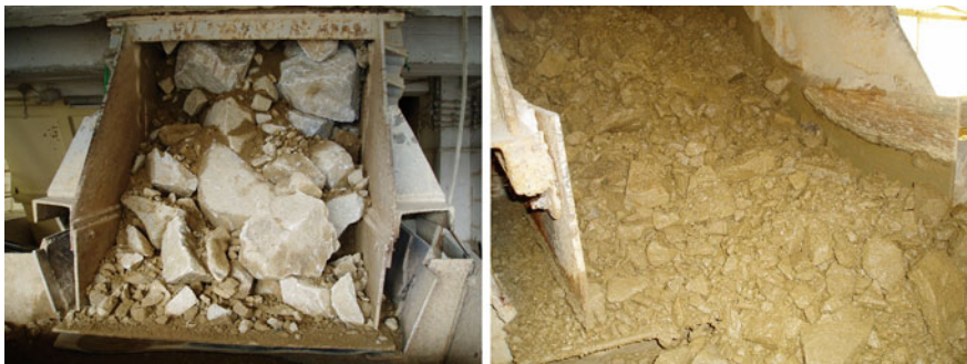
Fig. 3.5 Feeding material for autogenous milling; coarse fraction left and fine fraction (wet) right
