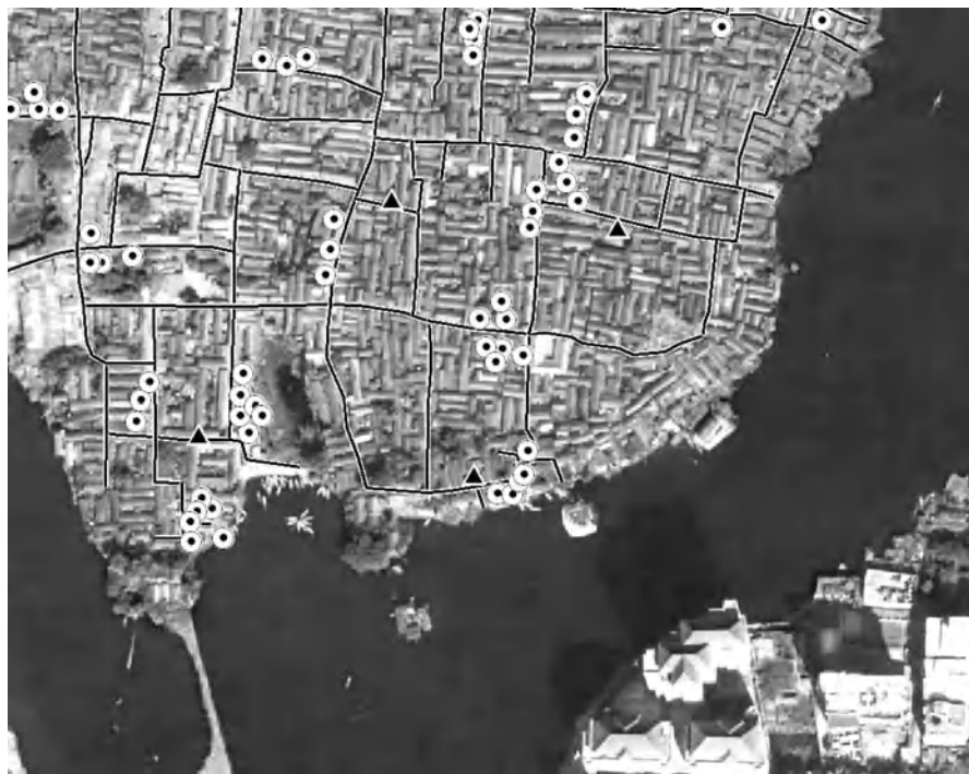
Fig. 10.2 Vector layer of wells ( triangles ) and GPS-based health survey locations (points: interviewed households) overlaid on satellite raster image of a slum in Dhaka, Bangladesh
