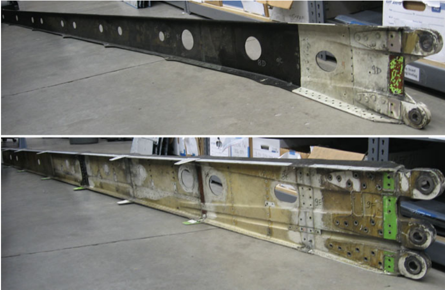
Fig. 13.16 R/H B-737 composite stabilizer spars – front spar ( top ), rear spar ( bottom )
