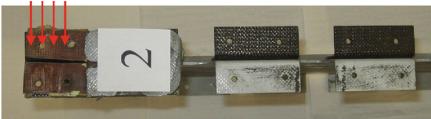
Fig. 13.18 Degradation of Tedlar ® , moisture barrier film
