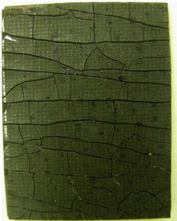
Fig. 2.9 Surface of PI + 40 wt% \text{Al}_2\text{O}_3 + 10 wt% fumed silica + 5 wt% carbon nanofiber after 200 h @ 316°C. Sample is a 1" square specimen
