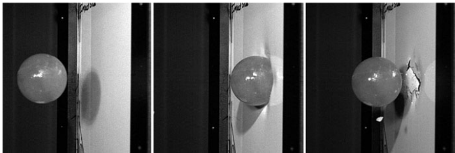
Fig. 5.23 High-speed video stills showing 61 mm ice impacting carbon/epoxy sandwich panel at 35 m/s producing localized damage to impact-side facesheet and core crushing; Note: ball stopped and rebounded by back-side facesheet
