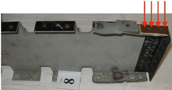
Fig. 13.19 Phenolic shims used to fill the gaps between the upper skin and ribs 2 and 8
