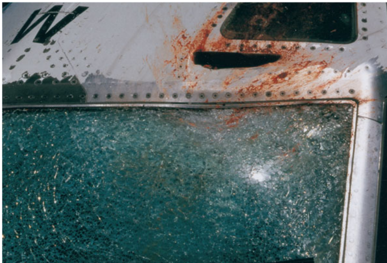
Fig. 5.14 Penetration damage to boeing 737 by bird impact at 10,000 ft altitude and 250 Kts causing injury to pilot (colour plate 11 [71])
