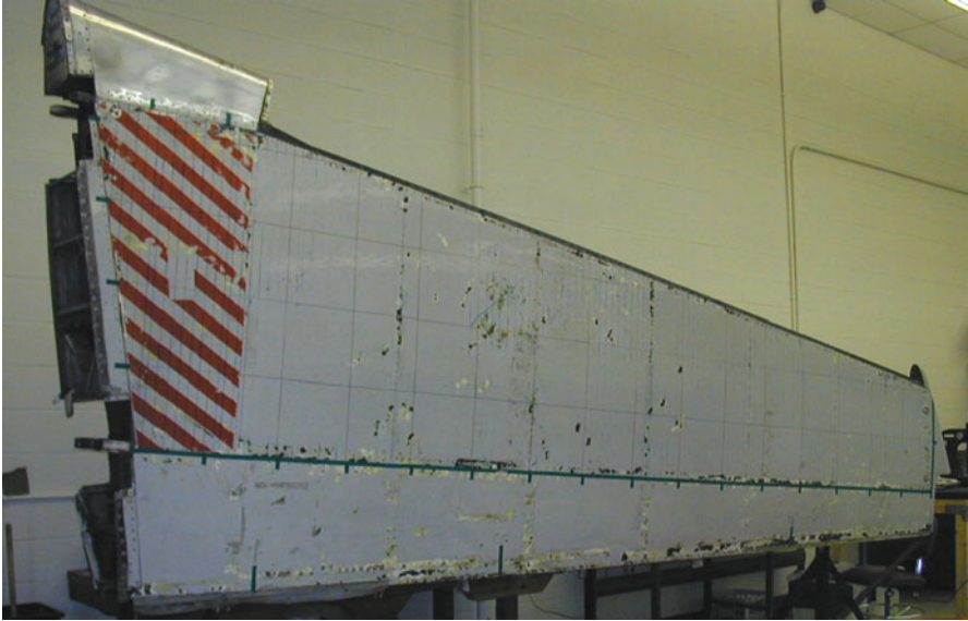
Fig. 13.10 B-737 CRFP R/H horizontal stabilizer prior to disassembly
