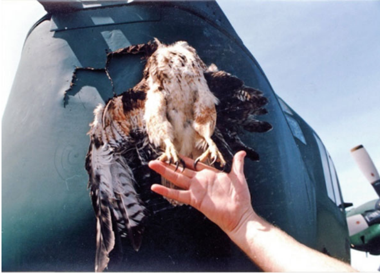
Fig. 5.11 Damage to nose cone of C-130 due to bird strike (USAF public domain photo)
