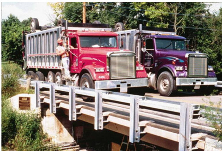
Fig. 16.4 Load testing using two trucks
