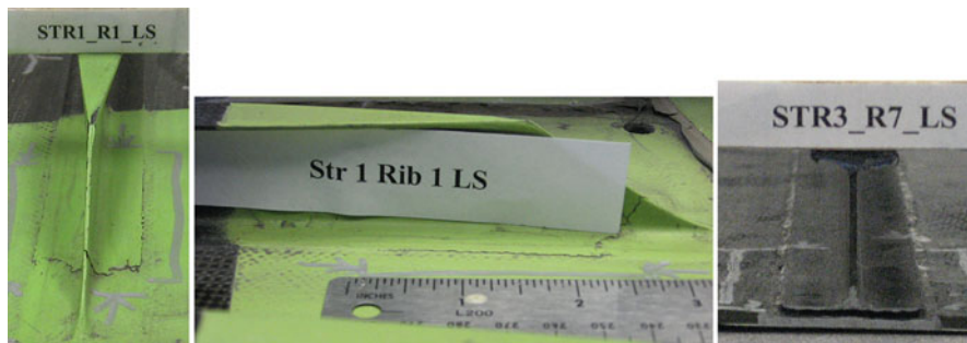
Fig. 13.22 Lower-skin disbonds confirmed after teardown
