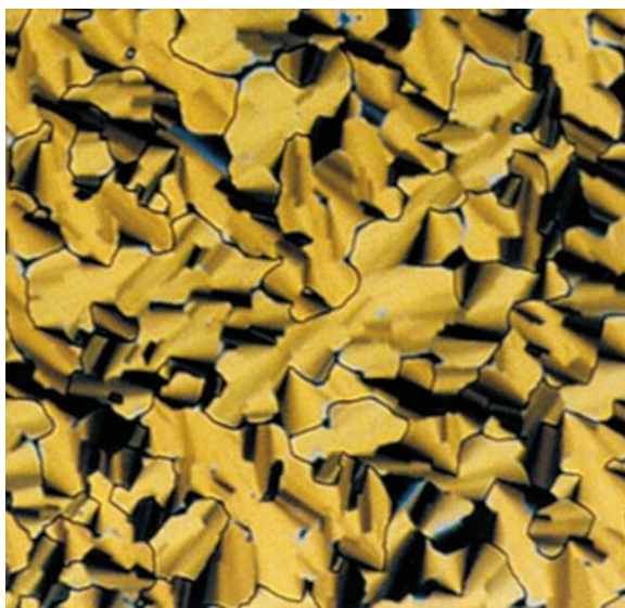
Fig. 20 Polarized light optical micrograph of the Col h phase of 134b at 103 °C. Reproduced by permission of The Royal Society of Chemistry from [127]
