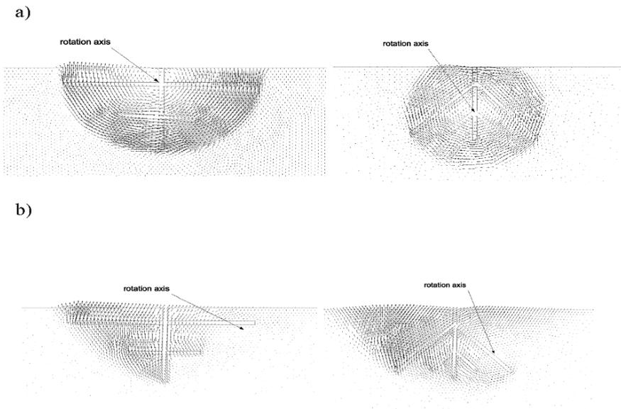
*Figure 4-9.* Numerical simulations of uprooting of two types of simple root architecture in a) clay-like soil and b) sandy-like soil. The displacement field in soil at the end of the uprooting simulations is shown. The point about which the root system rotates (rotation axis) is shown. The root-soil plate is more circular in clay-like soil compared to sandy-like soil, regardless of root system type (image courtesy of T. Fourcaud, see Fourcaud et al. 2007).
