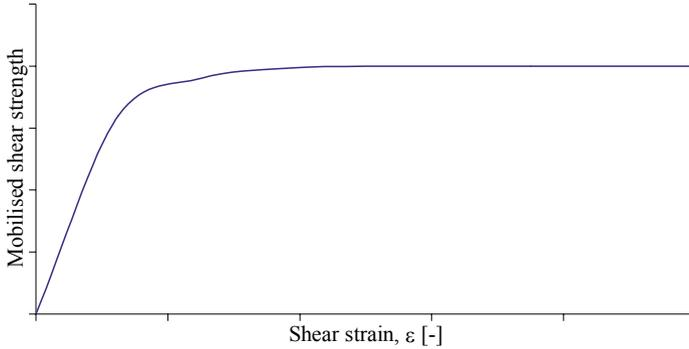
Figure 3-2. Material with constant stress-strain behaviour.
