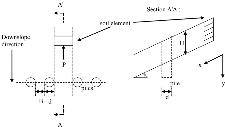
Figure 4-11. Soil arching action around a row of piles (redrawn from Wang and Yen 1974).
