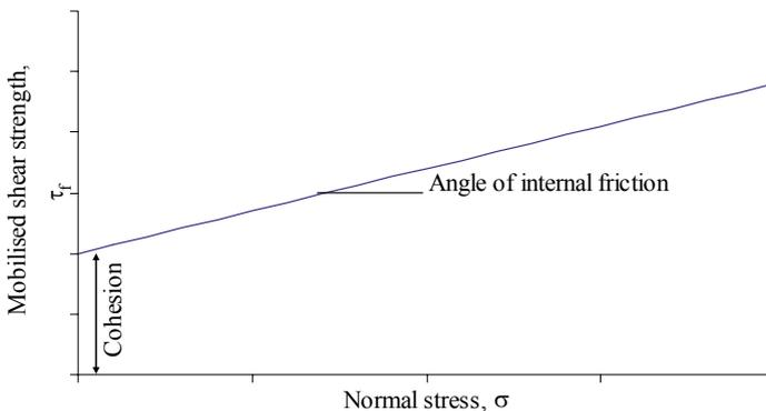
Figure 3-1. Mohr-Coulomb failure envelope.
