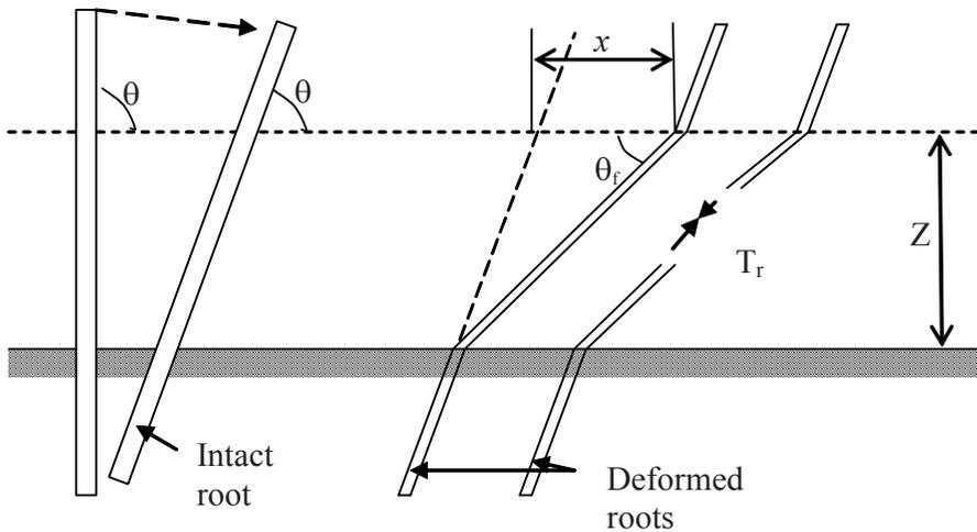
Figure 4-12. Root reinforcement model for perpendicular and inclined roots (modified from Gray and Leiser 1982).  $Z$  = shear zone,  $x$  = shear displacement,  $\theta$  = initial angle of intersection with shear plane,  $T_r$  = tensile strength of root,  $\theta_r$  = angle of intersection after deformation.
