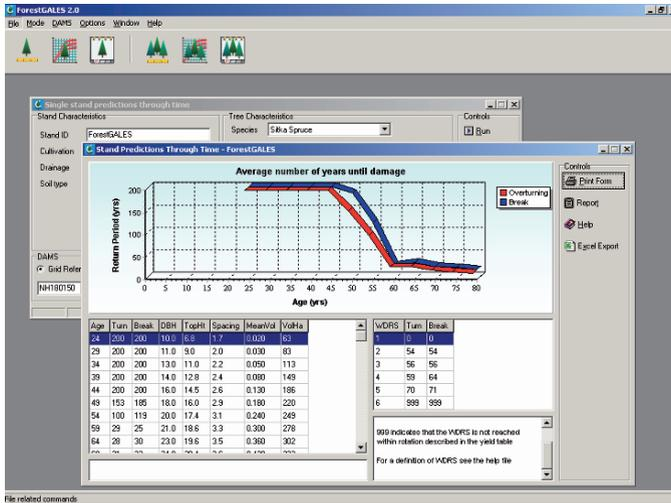
Figure 5-17. Example output screen from ForestGALES with the calculated return period displayed in the graph. Illustration courtesy of the Forestry Commission, UK.
