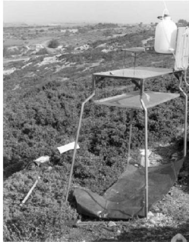
Figure 5-14. The drip-plate rainfall simulator (Amsterdam-type. Photo: E. Cammeraat).
