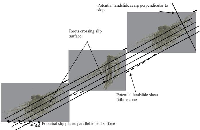
Figure 6-2. Roots crossing potential slip planes and shear surfaces will reinforce the slope against landslides (after Danjon et al. 2007, reprinted by permission of the publisher).
