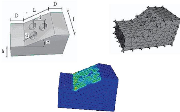
Figure 4-13. Example of 3D FEM model of slope stability with tree root inclusions (image courtesy of NM Kokutse, see Kokutse et al. 2006).
