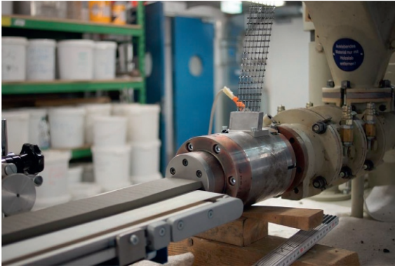
Figure 3.15 Extrusion with feeding device for textiles.
