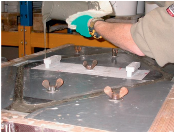
Figure 3.2 Casting the diamond-shaped element made of textile-reinforced concrete.
