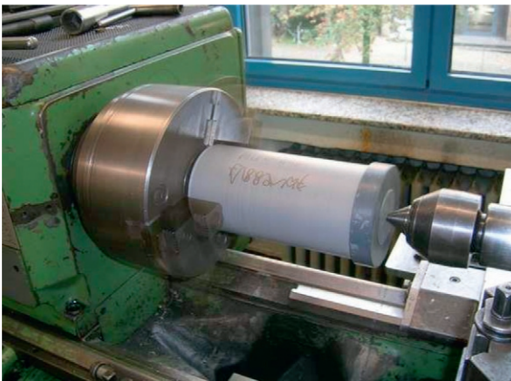
Figure 3.11 Clamped tube during the spinning process.
