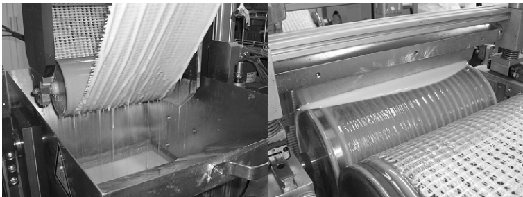
Figure 1.18 Ongoing coating process with an opened foulard (left) and a squeezing roller (right).
