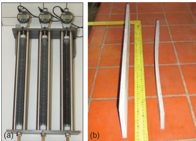
Figure 2.4 (a) Setup for testing autogenous shrinkage; (b) effect of shrinkage on TRC specimen cast with both surfaces facing the formwork (left specimen) and just one surface facing the formwork (right specimen).
