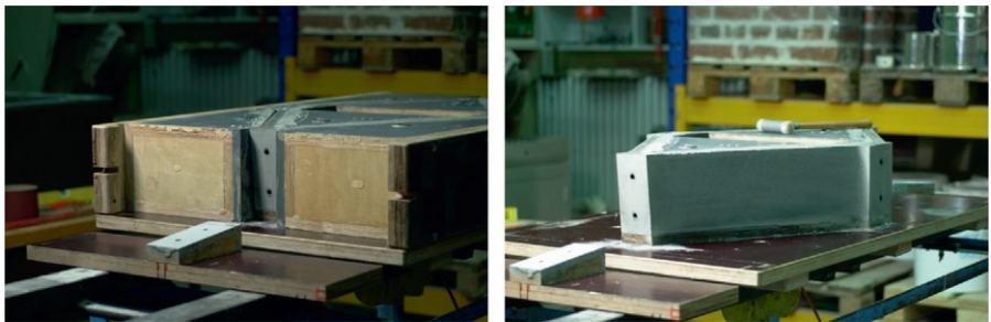
Figure 3.3 Demolding the diamond-shaped element made of textile-reinforced concrete.
