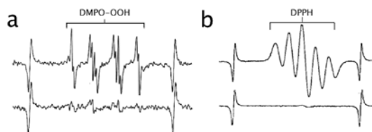
Figure 1. a. 0 ppm of PtNCs (an upper signal), 10 ppm of PtNCs (a lower signal). b. 0 ppm of PtNCs with hydrogen (an upper signal), 1 ppm of PtNCs with hydrogen (a lower signal)
