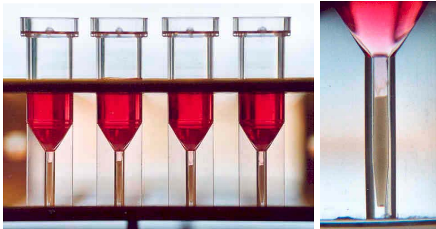
Figure 1. Prototype PCV microtube. The depicted tube is manufactured from transparent polystyrene. The capillary has a volume of 5 \mu l. A graduated scale for easily reading the PCV will be printed onto the tubes. Left: 2 samples in duplicate. Right: A sample with 3.6 \mu l of packed cells corresponding to 1.6 million CHO cells.
