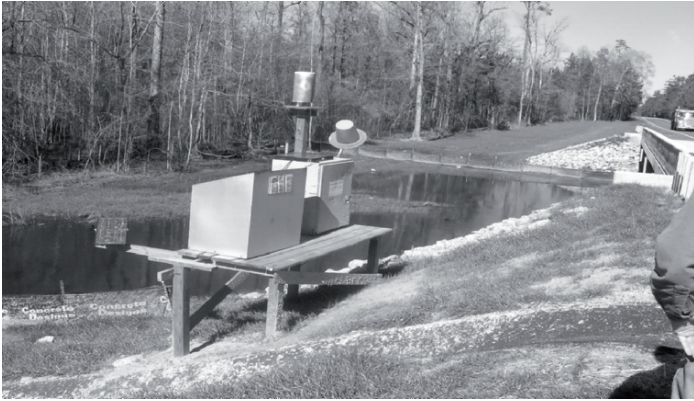
Figure 5. ISCO water quality sampler (front) connected with the USGS real time rain/flow recording Sutton datalogger (back).
