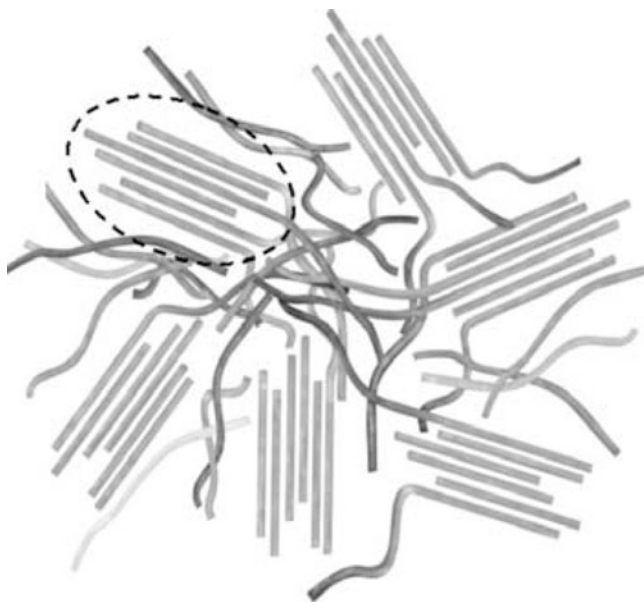
Fig. 6.2 The structure of the fluorocarbon polymer showing crystalline and fixed charges (the dotted lined circle indicates the crystalline of the fluorocarbon polymers) (Reproduced from Ref. [2] with kind permission of © Elsevier (2004))
