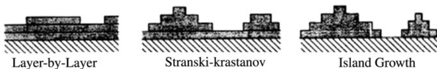
Fig. 1.9 The three most common growth modes. 2D layer-by-layer (Frank-van der Merwe type) growth, A 2D monolayer followed by 3D growth (Stranski–Krastranow) and 3D island growth (Volmer–Weber type)
