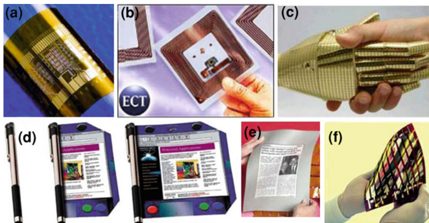
Fig. 1.1 Organic electronic devices a flexible circuitry from ECT inc, b flexible radio frequency identification tag, c flexible pressure sensors made using organic transistors from Univ. of Tokyo, d concept of a flexible display from ECT, e prototype flexible electronic paper from Plastic Logic, f , a flexible organic solar cell from Konarka Inc.
