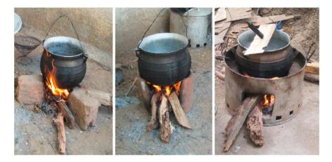
Fig. 11.1 Different wood stove models tested in the study (3-stone fire, ceramic stove and centrafricain stove)
