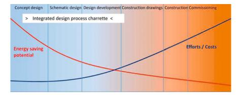
Fig. 16.3 Relationship between energy saving potential and costs in a building design process
