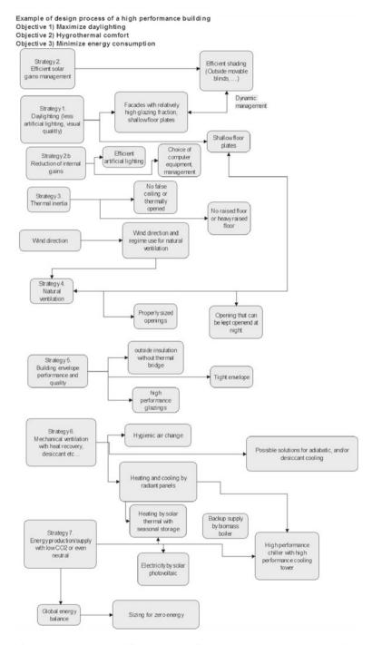
Fig. 16.4 Interactions between different energy efficiency strategies on a given building project
