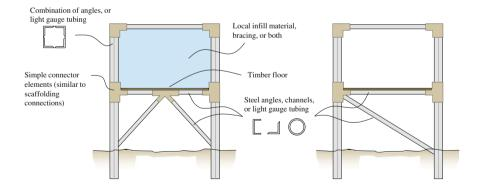
Fig. 19.7 Example multi-purpose element shelter configurations
