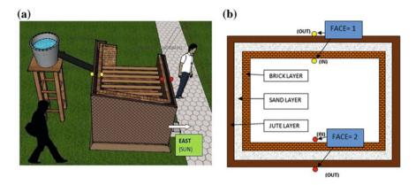
Fig. 9.1 RCS design configurations (schematics), (a) Conceptual diagram of jute model, (b) Schematic diagram of jute model
