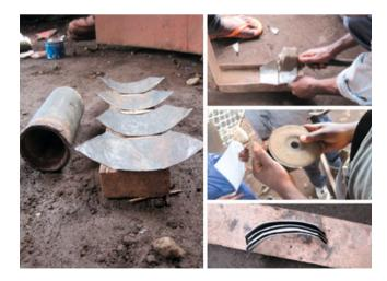
Fig. 5.5 Blade forming (Ho-Yan 2011d)
