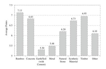
Fig. 19.4 Example LCA results per construction category (Reprinted here with kind permission Wallbaum et al. 2012)
