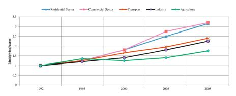
Fig. 16.2 Increase in final electricity consumption per sector since 1992
