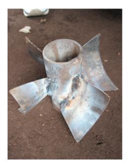
(Fig. 5.8). The weldments were inconsistent in length, and discontinuous along the seams. Excessive porosity and weld splatter are seen on some portions of the welds.
