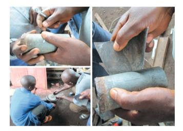
Fig. 5.6 Blade placement (Ho-Yan 2011e)
