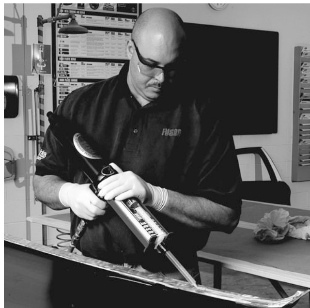
Fig. 14.6 Applying Fusor™ adhesive for repair of a steel automobile hood (Courtesy of Lord Corporation)
