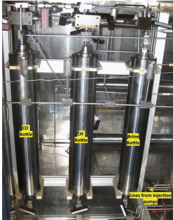
Fig. 3.4 Three fluid sample bottles containing the pressurised injection fluids
