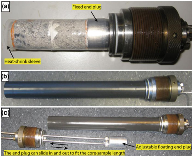
Fig. 3.19 a composite core sample placed inside a heat-shrink sleeve and the fixed end plug is inserted into one end of the sleeve. b The core-sample (after being wrapped in the aluminium foil) together with the fixed end plug are inserted into a long Viton sleeve. c The fixed end plug inserted into the sleeve assembly containing the core-sample beside the adjustable floating end plug
