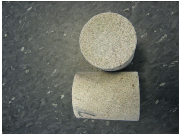
Fig. 3.14 Two glauconitic sandstone core-plugs drilled from whole-cores taken from an Australian gas reservoir—green dots are glauconite particles within the sandstone texture
