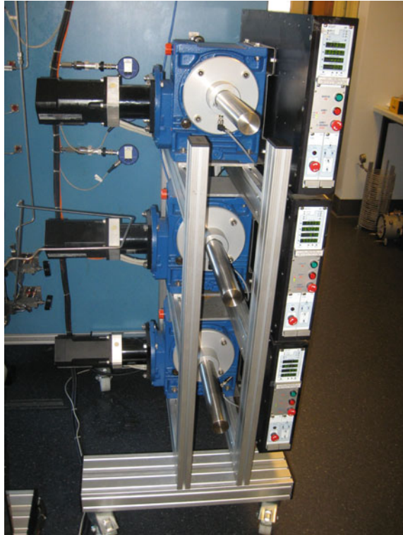
Fig. 3.9 Three collection pumps connected to the separator and their associated electronics
