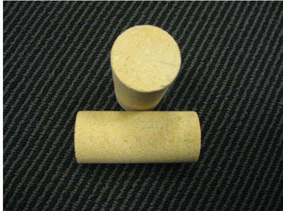
Fig. 3.13 Two Donnybrook Sandstone core-plugs taken from quarried blocks
