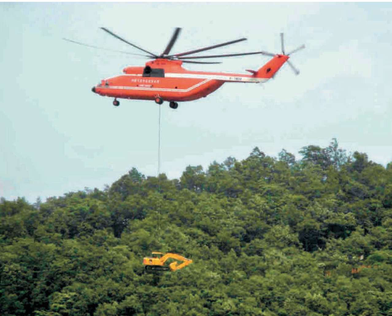
Figure 1.46 This Mi-26T heavy lift helicopter was used to bring heavy (13 tonnes) earthmoving tractors to the affected location (photo by Cai Yang, Xinhua News Agency).
