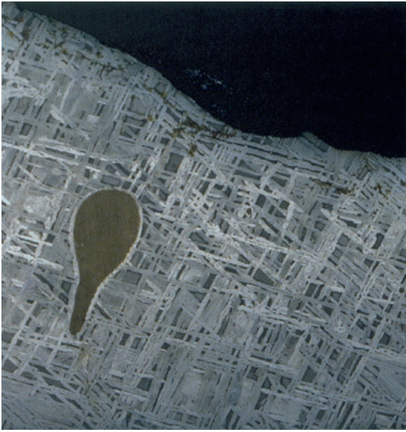
Fig. 18.3 Iron meteorites have a characteristic texture which appears on polished and etched surfaces. This texture, called the Widmanstätten pattern, formed during slow cooling and crystallization of liquid iron-nickel in the core of a meteorite parent body. The tear-shaped inclusion is composed of iron sulfide which is immiscible in iron-nickel liquid. The meteorite in this image is Carbo, a IID iron meteorite, which was not collected in Antarctica (Reproduced by permission of H. Haack from Haack and McCoy (2005, Fig. 8, p. 337) and Elsevier, Inc. through the Copyright Clearance Center, Inc., 222 Rosewood Drive, Danvers, MA 01932)
