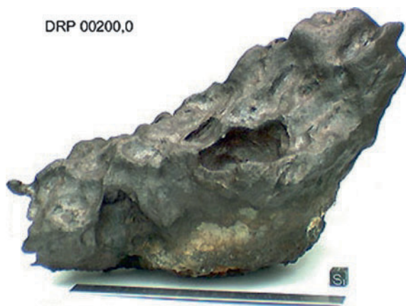
Fig. 18.22 This specimen of the Derrick Peak iron meteorite has a mass of 10 kg and is highly corroded as a result of chemical weathering after it fell about 1 million years ago. The upper surface is dark brown in color and is characterized by protruding crystals of schreibersite [(\text{Fe},\text{Ni})_3\text{P}] which are more resistant to chemical weathering than kamacite (Fe-Ni alloy). The original fusion crust and heat-altered surface layer are no longer present. The Derrick Peak meteorite is a member of group IIAB (coarse octahedrite) (Courtesy of NASA, JSC, Houston, Texas)
