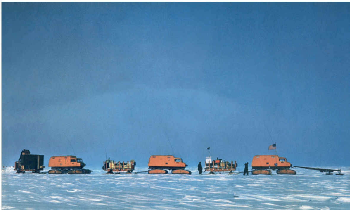
Fig. 2.18 The tractor train of the Marie-Byrd-Land oversnow traverse left Byrd station in West Antarctica on November 1, 1958, as part of the exploration of Antarctica during the IGY. The tractor train consisted of three Sno-cats each of which pulled a sled. The leading tractor, which was driven by Willam E. Long, carried a crevasse detector that projected from the front of the
