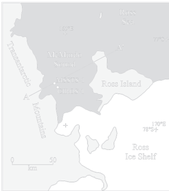
Fig. 19.1 CIROS-1 and MSSTS-1 in McMurdo Sound were drilled in order to recover cores of the sediment that would reveal the history of glaciation of the Transantarctic Mountains in southern Victoria Land during the Cenozoic. A third core (CIROS-2) was drilled a short distance in front of the floating ice tongue of the Ferrar Glacier (not shown). CIROS-1 reached a depth of 702 m ending in beds of sand and conglomerate dated at 36.2 Ma (Eocene) (Adapted from Barrett et al. 1989)
