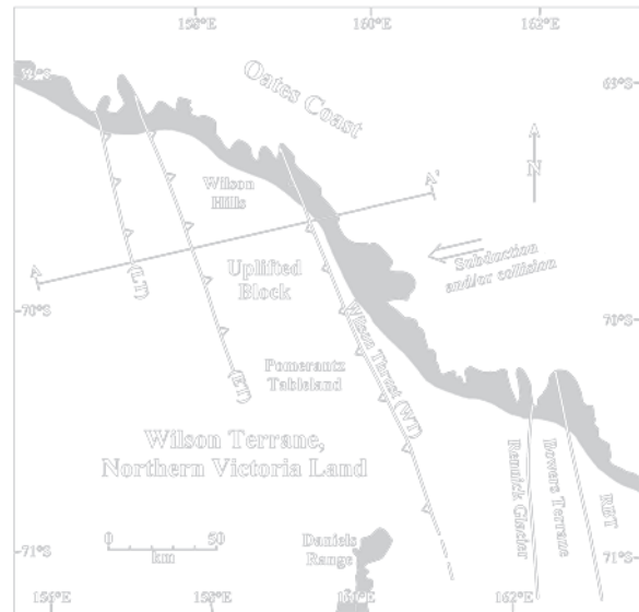
Fig. 4.28 The Wilson Terrane of northern Victoria Land (NVL) contains three thrust faults which define a crustal block that was uplifted as a result of compression from the east. The plane of the Wilson Thrust (WT) dips west at about 30° while the Exile Thrust (ET) and the Lazarev Thrust (LT) dip east. The uplifted block includes the Wilson Hills and the Pomerantz Tableland. The compressive force that activated the thrust faults originated either from the westward subduction, or by the collision of “suspect” terranes (i.e., BT and RBT) with the Wilson Terrane or both (Adapted from Adams 2006)
