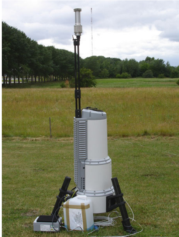
Fig. 3.13 Beam-focussing Doppler wind LIDAR. The laser beam is sent and received through the slanted top of the grey upper part of the main instrument. The small mast to the left carries the wind direction sensor
