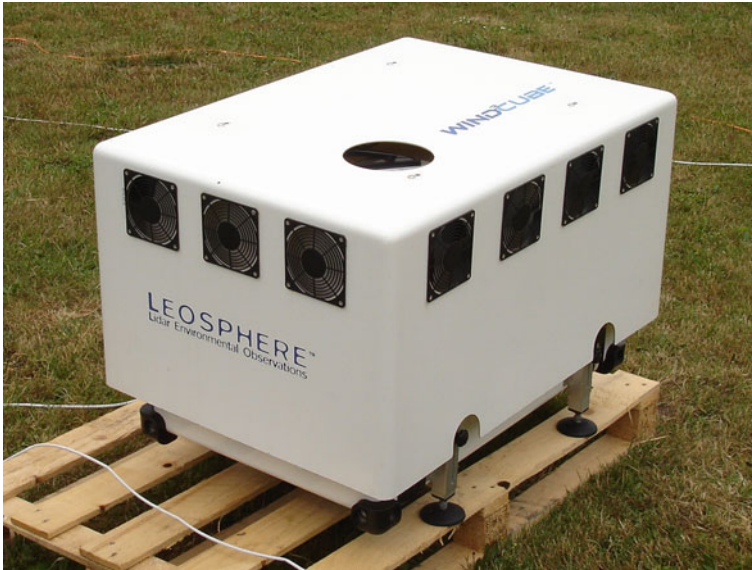
Fig. 3.11 Coherent Doppler wind LIDAR for wind energy assessment. The scanning infrared laser beam is sent (and the backscatter is received) through the circular opening on the top side of the instrument
