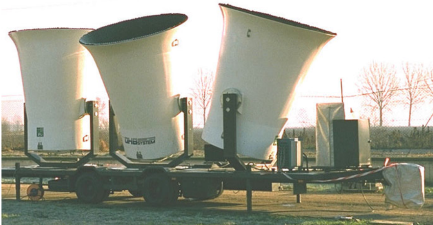
Fig. 3.4 Three-antenna sodar for wind and turbulence profile measurements up to about 1000 m above ground
