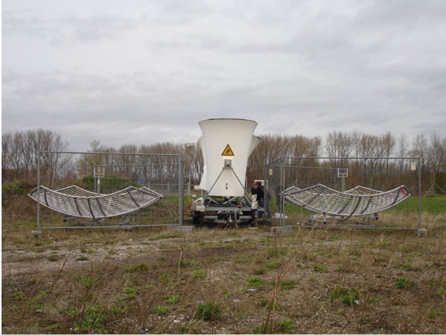
Fig. 3.8 Radio-acoustic sounding system (Sodar-RASS) for profile measurements of wind, turbulence, and temperature. The acoustic sounder (sodar) with its three white antennas is in the middle, the emitting radio antenna is to the left and the receiving radio antenna is to the right
