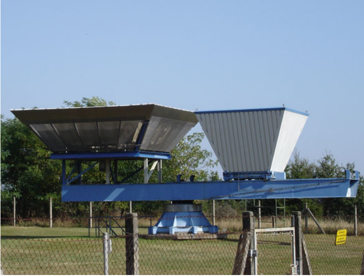
Fig. 3.2 Boundary layer wind profiler of the German Weather Service at the Richard Aßmann observatory in Lindenberg. The electromagnetic antenna is to the left , the acoustic sound source to the right
