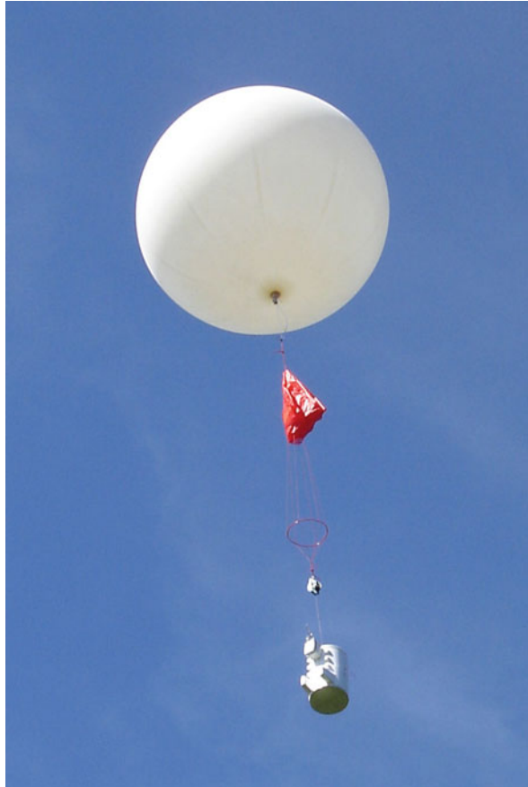
Fig. 1.3 Balloon carrying an ozone sonde just after launching from the Hohenpeissenberg observatory of the German Weather Service
