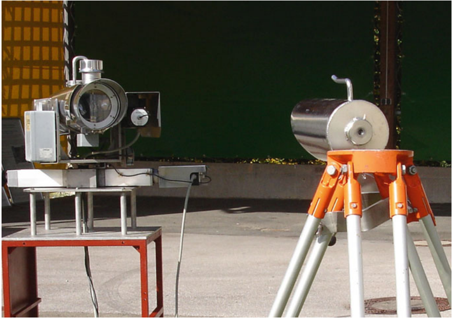
Fig. 3.15 DOAS instrumentation for open-path trace gas concentration measurements. Left : light source and receiving telescope, right : mirror. In operation the two parts are installed several hundreds of metres apart
