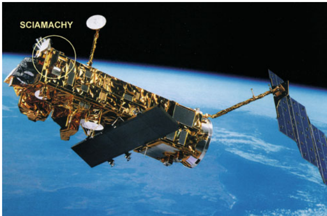
Fig. 2.1 Artist's impression of ENVISAT in orbit. SCIAMACHY is located at the upper right corner of the payload front panel (Photo: ESA).
