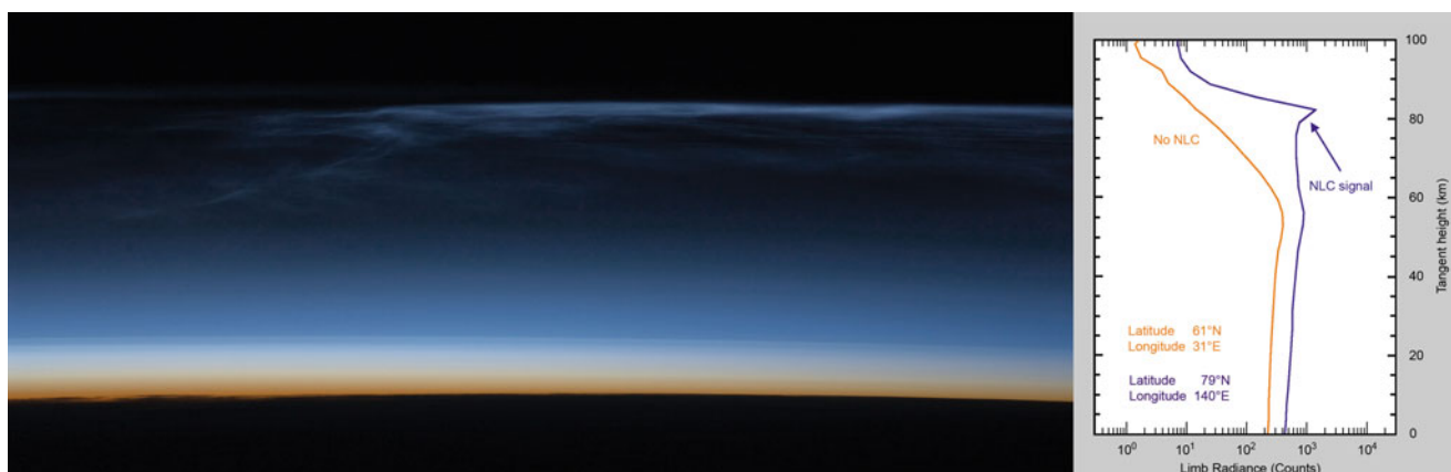
Fig. 10.30 NLC as seen from the International Space Station on 22 July 2008 ( left panel ) together with the NLC signature in a SCIAMACHY UV limb radiance profile from 3 July 2002 ( right panel ). The scattering by ice particles in the NLC leads to a significant increase of the observed limb radiance profile peaking at the characteristic NLC altitude of about 83–85 km ( blue line ). Shown in red is for comparison a limb radiance measurement without NLC being present (Courtesy: C. von Savigny, IUP-IFE, University of Bremen; ISS photo: NASA).
