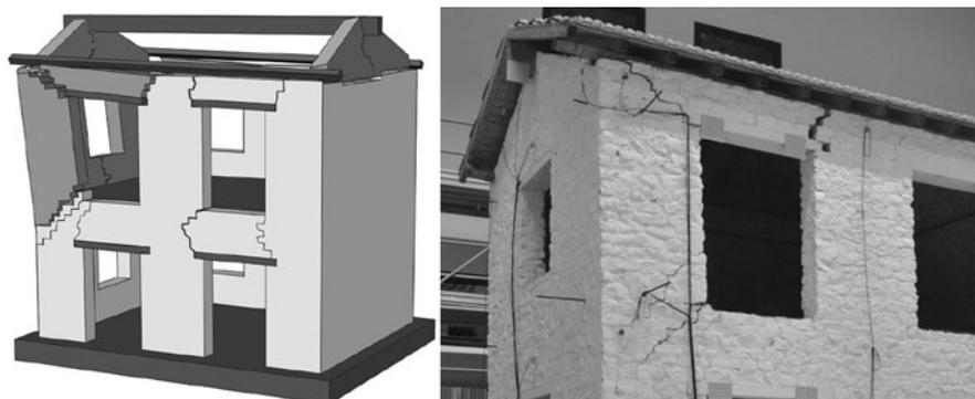
**Fig. 8.3** Observed collapse mechanism during the shaking table test of a full-scale stone masonry building with flexible floors, without tie-rods (Magenes et al., 2010)
