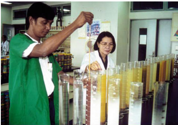
Fig. 1.27 The field textural observation is usually confirmed in the laboratory using either Bouyoucos hydrometer method or the pipette method. The results are compared with the soil textural triangle for final textural classification
