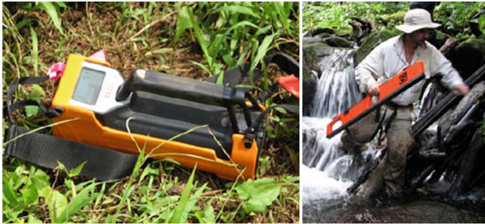
Fig. 1.18 a and b Emerging technique in soil survey is rapid measurements in the field, although less precise is compensated by many sampling points. In the BSWM-ACIAR project for mapping of Cabulig watershed, two instruments were tested—gamma radiometrics
