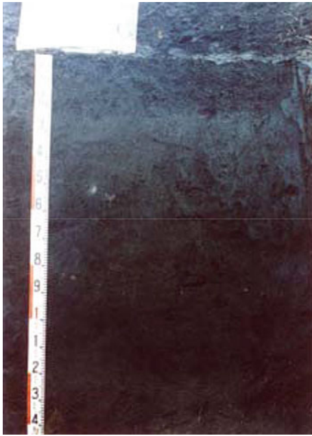
Fig. 4.3 Soil profile of tephra-derived Mayon series with the melanic epipedon and greasy feel characteristics of the more commonly known Andisols
