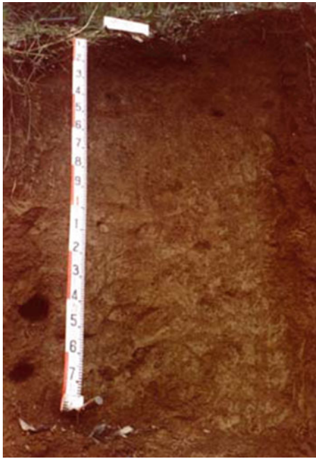
Fig. 1.21 An Oxisol soil profile; the presence of an argillic horizon or movement of clay into the lower layer, is a prerequisite for classifying Mollisols, Alfisols, Ultisols, and Oxisols. This can be confirmed by textural analysis in the laboratory
