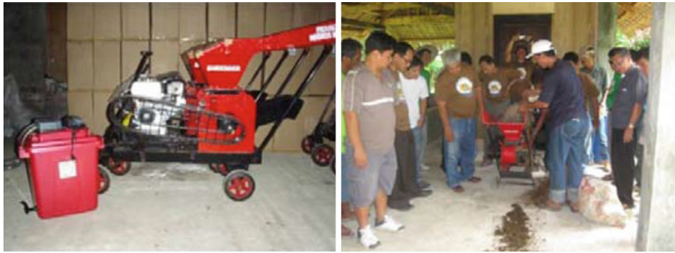
Fig. 5.7 Left Set of tea brewer and shredder distributed to farmer groups and organizations for community-based production of organic fertilizers as part of the national government food production program
