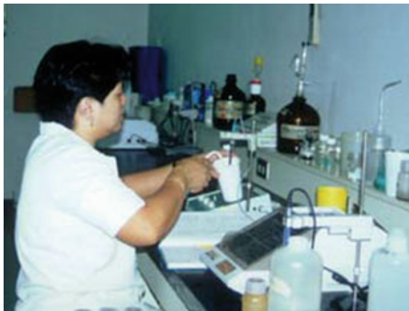
Fig. 1.34 Field obtained pH value is further validated in the laboratory using more precise pH meter and presented as part of the chemical–physical laboratory analysis of the soil samples
