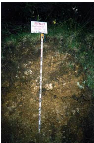
Fig. 1.39 Soil profile of Faraon series, developed from sedimentary rocks. Limestone soils do not follow the substratum characterization and are classified according to soil color. Faraon soils belong to black or dark colored soils
