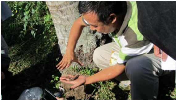
Fig. 1.30 Soil consistency is the strength soils resist fragmentation, deformation and rupture, usually described at either dry, moist, or wet moisture state. In the field this is usually measured in terms of stickiness (how the soil particles adhere to fingers after release of pressure) and plasticity (evaluation done by forming a 4 cm long wire of soil at a water content where maximum plasticity is expressed)
