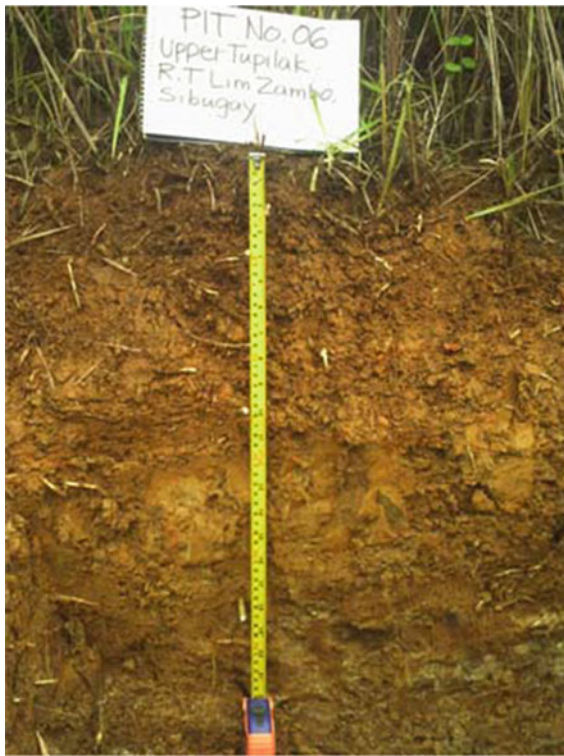
Fig. 1.13 We observe a two-dimensional soil profile through a purposive pit digging and assume this to be a representative of a three-dimensional basic unit of soil, the pedon
