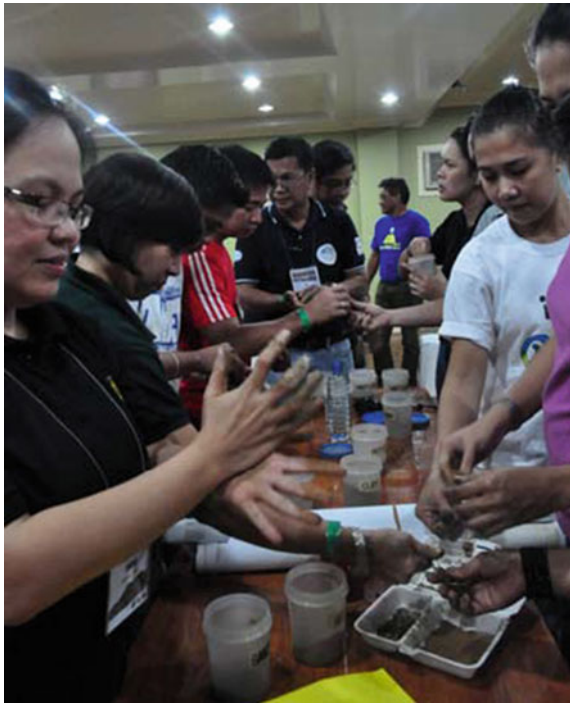
Fig. 1.26 Soil texture by feel method is not hit and miss proposition. Determining soil texture by feel method can be studied using soils with predetermined soil texture. One starts with mastering how loamy soils feel and imagine this as the center of the textural triangle; the soil becomes more clayey as we move to the upper corner; more sandy as we move to the lower left corner; and more silty as we move to the lower right corner of the textural triangle
