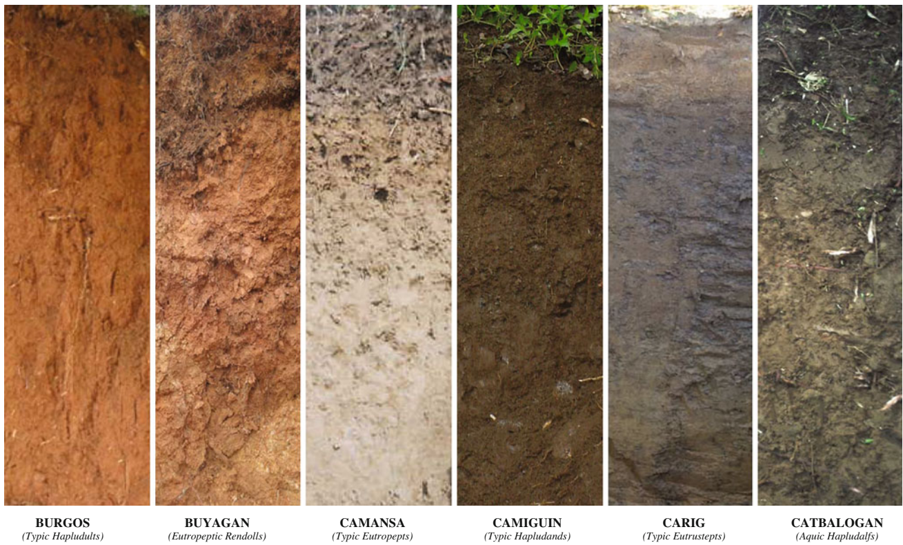
Plate 3C Soil profiles of Burgos, Buyagan, Camansa, Camiguin, Carig, and Catbalogan series. Highland and mountain soils of the Philippines (Photo credit BSWM and UPLB)
