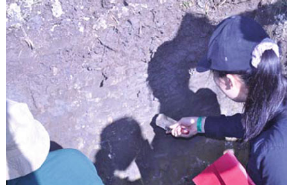
Fig. 1.32 The first part of the pit protocol is horizonization, determining and measuring the horizon boundaries
