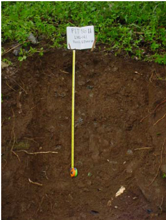
Fig. 1.82 Typical pedon of Camiguin series characterized by presence of big boulders of basalt and andesite as well as rock outcrops scattered in abundance on the surface soil. In classical soil survey, sampling is done purposively
