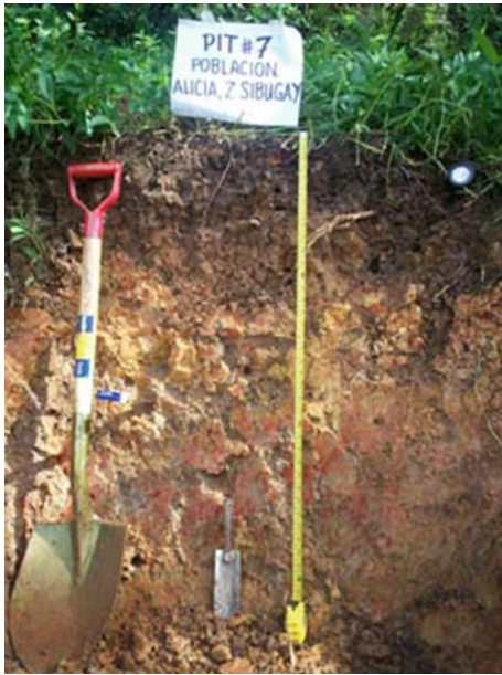
Fig. 1.22 A soil profile characterized by presence of plinthite is amazingly colorful because of the reddish color that the concretionary ironstone imparts to the visual sense. But these soils are difficult to work with because of the limiting root zone
