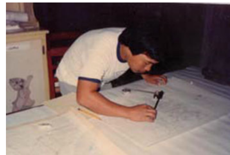
Fig. 1.17 Soil surveyors develop the landscape-soil relationship to be able to delineate soils in the map. Classical soil surveyors compute the area coverage using traditional tool like a planimeter. In today's post soil survey activities, computer-assisted GIS tools facilitate area computation. The use of satellite images also enhance landscape studies
