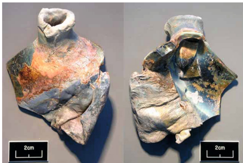
Fig. 1 Opalescent glassworking waste. Eighteenth-century wine bottle waster from Limekiln Lane, Bristol, UK (sample 4)
