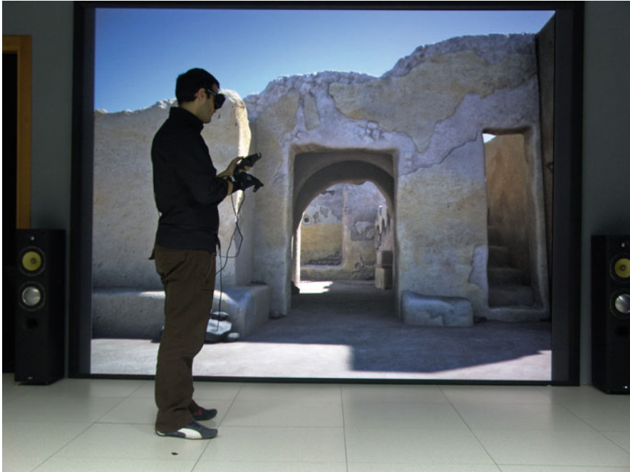
Fig. 2 User wearing wireless trackers and stereoscopic goggles during navigation through the reconstructed environment
