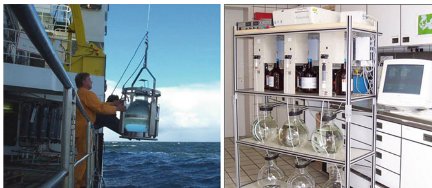
Fig. 19.3 Glass bowl sampler for 100 L ( left ) and SPE system for 1–30 L ( right ) water samples
