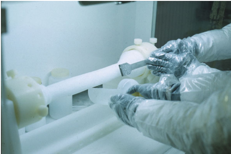
Fig. 3.4 Decontamination of an ice core by chiselling veneer layers of ice in progression from the outside towards the center inside a laminar flow clean bench in a cold room (Photo C. Boutron)
