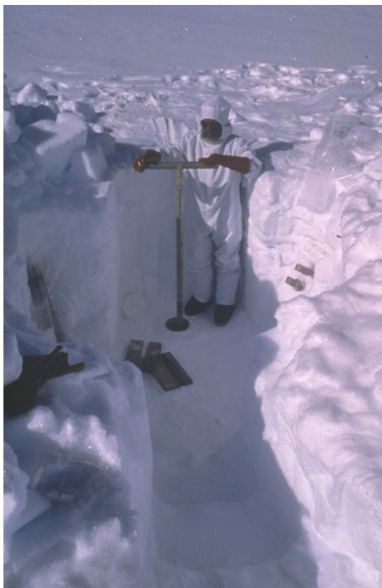
Fig. 3.3 Collection of a 10 m snow core in central Greenland (Summit) using an acid cleaned hand operated polycarbonate auger (Photo C. Rado)
