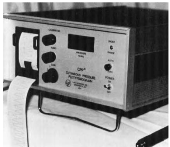
FIGURE 18-6 The cutaneous pressure plethysmograph.
