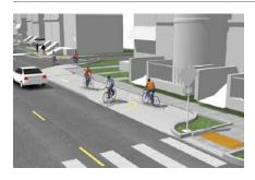
A **two-way cycle track** has the advantage of diverting bicyclists traveling in either direction on a bicycle boulevard to a single crossing location. This minimizes the cost of the crossing treatments and enables the use of beacons and signals, which cannot be used in close proximity.
