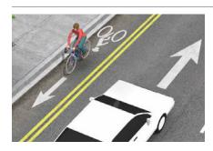
If the connecting street is one way for motor vehicle traffic, consider allowing bicyclists to travel against the flow of traffic using a contra-flow bike lane. **Contra-flow bike lanes** are installed on one side of the street facing one-way vehicle traffic.
