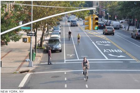
In a case study looking at the influence of pavement markings and bicyclist positioning, researchers found that, "the bicycle lane [with an edge line demarcating the parking lane] was the most effective at keeping cars parked closer to the curb and encouraging cyclists to ride in a consistent position at intersections."
