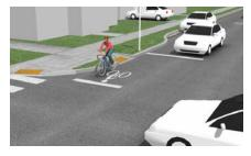
A **bicycle forward stop bar** can reduce the minimum acceptable gap by one second per side of the street.
