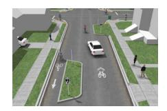
Chicanes are a series of raised or delineated curb extensions, edge islands, or parking bays on alternating sides of a street forming an S-shaped travel way. This reduces vehicle speeds by requiring drivers to shift laterally through narrowed travel lanes.<sup>138</sup>
