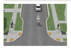
Neckdowns are pinchpoints at intersections; they are minor street crossing treatments that narrow at least one side of an intersection using curb extensions or edge islands on both sides of the street. They are often combined with parking bays on side streets off of commercial main streets.<sup>140</sup>
