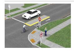
A **forced turn at an intersection** restricts through movements for motor vehicles. This diversion can exclusively use signs to allow buses and emergency vehicles to continue straight, but this may result in poor compliance by motorists (Berkeley, 2000).
