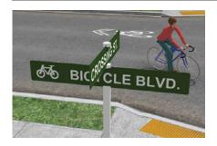
Modified street signs identify and brand the route without introducing a new sign. A bicycle symbol can be placed on a standard road sign, along with the coloration associated with the bicycle boulevard network. These are commonly used in tandem with pavement markings.
