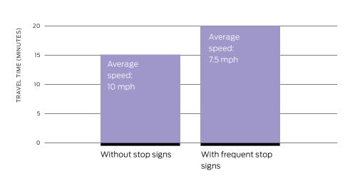
Calculations assume a 2.5 mile trip distance. Delay calculation adapted from: City of Berkeley. (2000). Bicycle Boulevard Design Tools and Guidelines.
