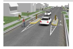
A pinchpoint or choker narrowing includes curb extensions or edge islands placed on either side of the street to narrow the center of the lane such that two drivers have difficulty passing through simultaneously. Pinchpoints should only be used where traffic speeds are already low. Cut-through passageways should be provided to the outside of the pinchpoint to accommodate bicyclists.<sup>139</sup>
