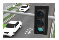
At an offset intersection where a signal exists, **signal phasing** can accommodate bicyclists riding through the intersection. This treatment will require a longer phase on the major street than a standard intersection, as it should provide sufficient time for bicyclists to travel through the jog.
