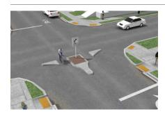
A channelized right-in/right-out island forces motor vehicles to turn right while bicyclists can continue straight through the intersection. The island can provide a through bike lane or bicycle access to reduce conflicts with right-turning vehicles.
