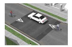
**Speed tables** are longer than speed humps and flat-topped, with a height of 3 to 3.5 inches and a length of 22 feet. Vehicle operating speeds range from 25 to 35 mph, depending on the spacing, and speed tables may be used on collector streets and/or transit and emergency response routes.
