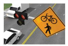
**Hybrid beacons** can facilitate bicycle crossing of a busy street where cross traffic does not stop but side street volumes do not warrant installation of a conventional traffic signal, or where a full traffic signal installation is not desired.
