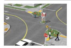
**Diagonal diverters** placed at a fourway minor intersection require all motor vehicle traffic to turn, while allowing bicyclist and pedestrian through movements.<sup>152</sup>
