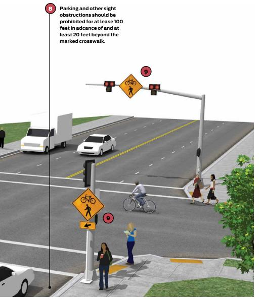
Parking and other sight obstructions should be prohibited for at least 100 feet in advance of and at least 20 feet beyond the marked crosswalk, or site accommodations should be made through curb extensions or other techniques to provide adequate sight distance.<sup>90</sup>
