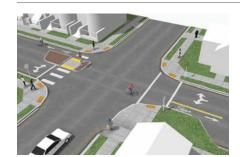
Partial closures or choker entrances across one direction of traffic at an intersection allow full bicycle passage while restricting vehicle access to one side only. Motorists on the bicycle boulevard must turn onto the cross street while bicyclists may continue straight along a short contra-flow bike lane past the closure.
