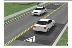
Split speed tables are also 22 feet long and extend across one direction of travel lanes from the centerline. A longitudinal gap is provided to allow emergency vehicles to weave around the treatment. While studies have indicated that this treatment does not reduce speeds below 25 mph, it has been found to deter cut-through traffic, particularly by large trucks.<sup>135</sup>
