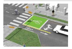
Signs that prohibit through movements, right-in/right-out splitter islands, and partial closures are volume management strategies to reduce cut-through motor vehicle traffic. Signs are typically less effective than physical diversion.
