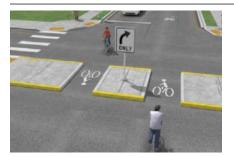
Median islands/diverters restrict through vehicle movements while providing refuge for bicyclists to cross one direction of traffic at a time (also see major street crossing treatments). A snake diverter is a narrow raised median that is an extruded curb along the centerline of the cross street. This treatment minimizes impacts for travelers on the cross street while prohibiting through movements by motor vehicles on the bicycle boulevard.
