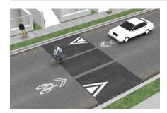
**Speed cushions** or speed lumps are either speed humps or speed tables that include wheel cutouts to allow large vehicles to pass unaffected, while reducing passenger car speeds. They can be offset to allow unimpeded passage by emergency vehicles and are typically used on key emergency response routes. They should be used with caution, however, as people driving sometimes seek out the space between the lumps, reducing the traffic calming effect and causing unpredictable driving.<sup>134</sup>
