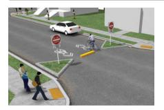
**Full diverters** create a "T" blocks motor vehicles from continuing on a bicycle boulevard, while bicycle travel can continue unrestricted. Full closures can be constructed to be permeable to emergency vehicles.
