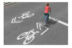
Pavement markings identify the route as a bicycle boulevard and can guide users through jogs. These vary throughout North America from small dots about a foot across to stencils that take up nearly a full lane at 30 feet by 6 feet. Several jurisdictions are using MUTCD-approved shared lane markings on bicycle boulevards for consistency with the rest of the bicycle network and because they are visible and proven to impact desired lane positioning by bicyclists.<sup>127</sup>
