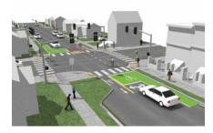
Bike boxes allow bicyclists to get to the head of the queue at signalized intersections. This allows them to take advantage of the typically short green time provided to the minor roadway at an intersection with a major roadway. Such boxes also increase bicyclist visibility to drivers. Parking removal should be considered where a bicycle boulevard has insufficient space to provide the ingress lane to a bike box.
