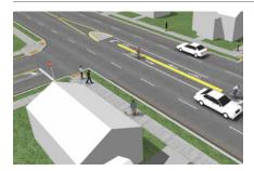
A **median island** is similar to the center turn lane treatment, except an extruded curb end cap provides more of a buffer than just paint. This type of crossing can be used to accommodate a jog in either direction, as bicyclists can cross one lane of traffic and ride in the median.
