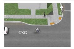
Curb extensions or bulb-outs extend the sidewalk or curb face into the parking lane at an intersection. When placed on the bicycle boulevard, they visually narrow the roadway. Curb extensions on the cross street act as a minor street crossing. All curb extensions reduce the crossing distance for pedestrians, can increase the amount of space available for street furniture and trees, and can act as stormwater management features.
