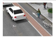
A pair of **one-way cycle tracks** can be used along the section of roadway connecting the offset segments of a bicycle boulevard. This treatment requires crossing treatments on both sides of the facility, and may facilitate wrong-way riding on the cycle track.
