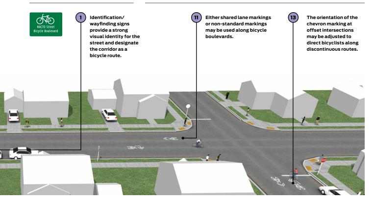
bicycle marking in the center of the roadway and two sets of chevrons offset 1 foot in each direction or travel.
