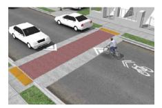
A raised crosswalk is a speed table that is marked and signed for pedestrian crossing. It extends fully across the street, can be longer than a typical speed table, and is typically 3 inches high. An entire minor intersection can be raised to reduce motor vehicle speeds in all directions.<sup>136</sup>
