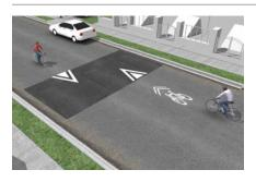
**Speed humps** are 3 to 4 inches high and 12 to 14 feet long, such that speeds are reduced to 15 to 20 mph. They are often referred to as "bumps" on signage and by the general public.<sup>133</sup>
