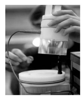
**Fig. 15.2** Electroporation of fish eggs. Eggs (15–50) are placed in a DNA solution inside the cuvette and then placed between two electrodes to receive rapid pulses of high voltage (Source: Dunham 2004)
