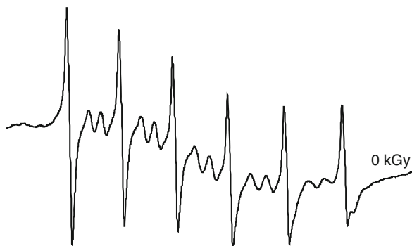
Fig. 8.4 EPR spectrum of sea shell of the family of Ostrea SP recorded before irradiation
