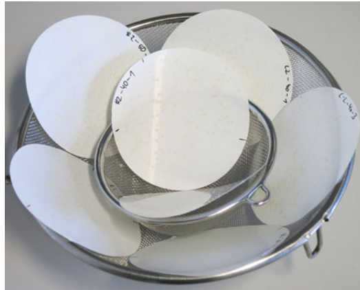
Fig. 3 Arrangement of the membranes on a mesh prior to cell permeabilization by chloroform vapor
