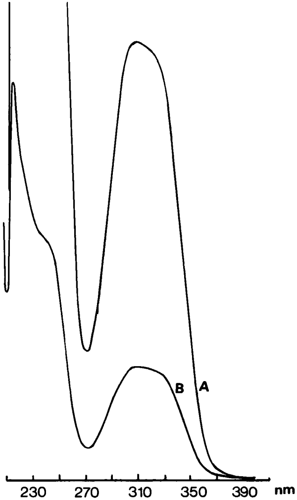
Figure 2. Ultraviolet Spectrum of Bromocriptine Mesilate in 0.1 M Methanolic Methanesulphonic Acid. C_A = 0.05 mg/ml, C_B = 0.012 mg/ml. Instrument: Philips SP 1700
