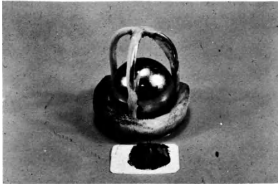
Figure 22.10 An example of very extreme cloth tear of the Model 2310 valve which was covered by two layers of Teflon
