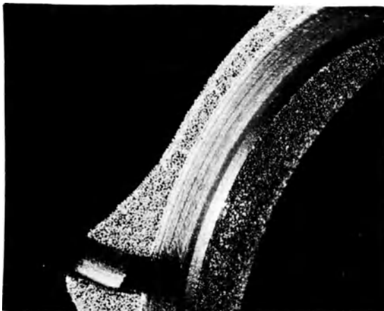
Figure 22.13 Metallic beads (highly magnified) plastered onto the surface of a prosthesis
