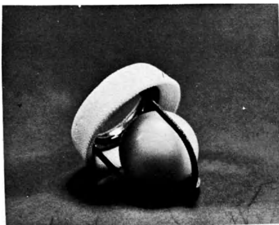
Figure 22.14 Model 1200, showing a metallic surface around most of the strut leaving a smooth inner track for the surface of the ball to impinge upon
