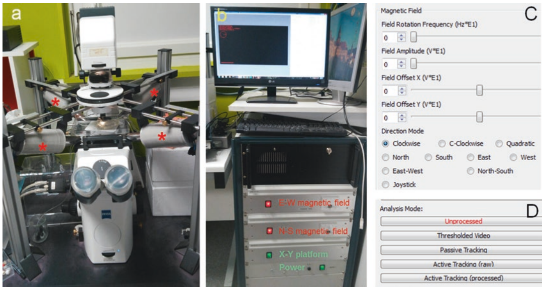
Fig. 2 The Magnetodrome system. Panel (a) shows Zeiss Axio Observer A1 microscope and the four electromagnets (stars). Panel (b) shows the MAGNETODROME controller with real-time display screen and the power control units of Magnetodrome system (Bottom with function marks). Panels (c) and (d) show the control panels of magnetic field and analysis mode of MAGNETODROME software, respectively
