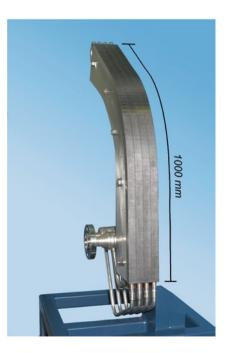
**Fig. 9.7** A water-cooled divertor test surface [31]
