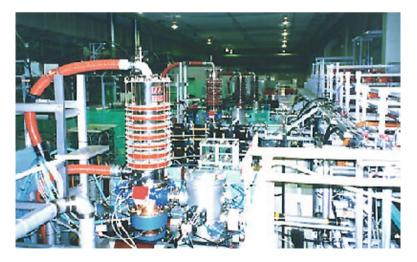
Fig. 9.24 The gyrotron room at JAERI [35]. A 1-MW gyrotron is shown at the *left*. It is 3 m (10 feet) high and covered with magnetic coils
