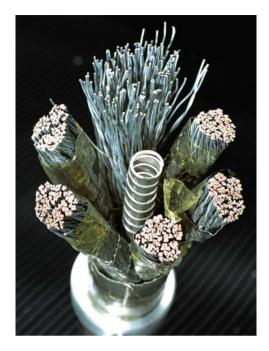
Fig. 9.21 Construction of a niobium-tin cable. One of the bundles has been exploded to show the strands [14]
