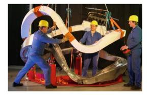
Fig. 10.4 Two Wendelstein 7-X coils [8]
