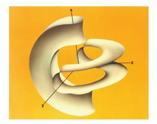
Fig. 10.22 Yin-yang coils (An old diagram or picture originally from Lawrence Livermore National Laboratory.)
