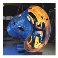
Fig. 10.5 A section of the Wendelstein 7-X vacuum chamber [8]
