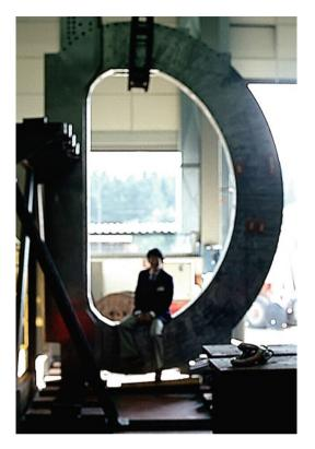
Fig. 7.12 A D-shaped ASDEX coil
