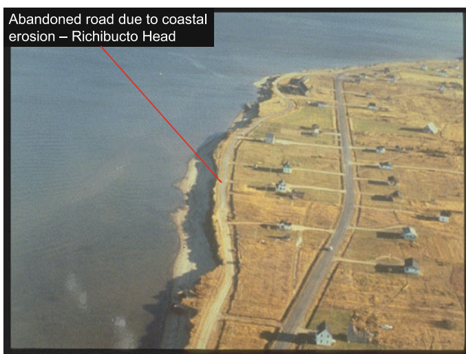
Fig. 2.17 Abandoned road due to coastal erosion at Richibuctou Head (Cap Lumière). Source New Brunswick Department of Environment/Paul Jordan
