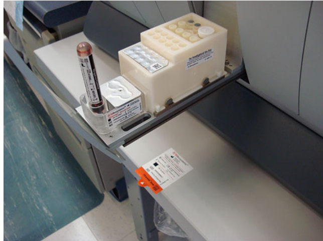
Fig. 9 Hold the T2 Candida panel in place after loading and gently pull off label. Place it on the counter under the drawer
