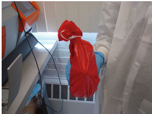
Fig. 12 Grab top of the bag, let go of the cartridge, and close bag with a twist tie
