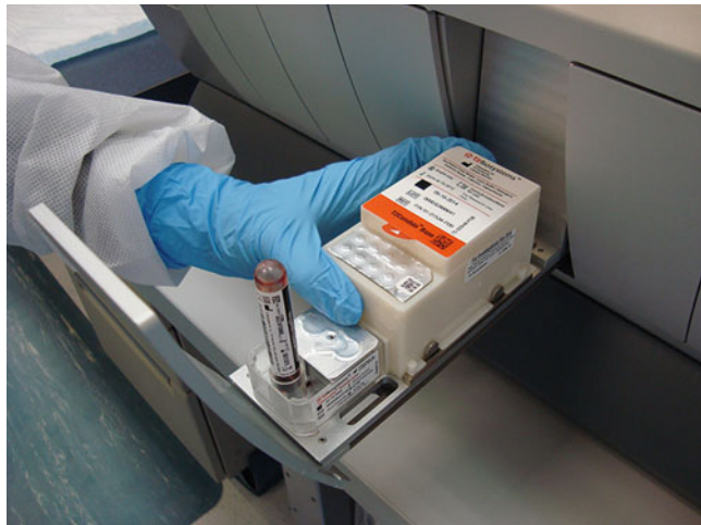
Fig. 8 Load the T2 Candida panel and without letting go, gently wiggle it in place to make sure it is seated properly and the posts are aligned
