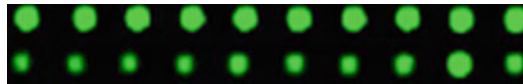
Fig. 4 Evaluation of spotting buffer. Two distinct spotting buffers were tested in spotting of fluorescently labeled amino-modified oligonucleotides on epoxy-coated slides. Slides were treated after spotting as described in Subheading 5.3. and scanned immediately afterwards
