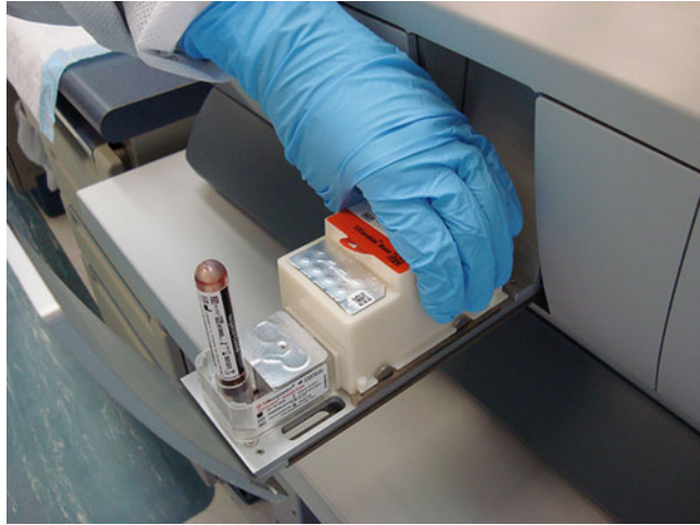
Fig. 7 Pick the assembled T2 Candida panel up by placing left hand over the top of the cartridge body and grabbing both sides of it or grab both ends of the cartridge body and place the little finger under it for stability
