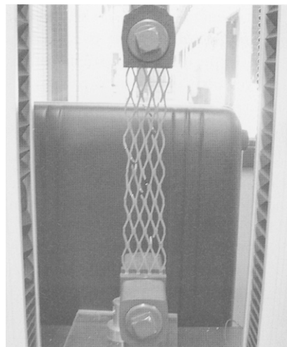
Fig. 9.15 Ribbon with a few strands punctured and severed by simulated meteorite impacts.
