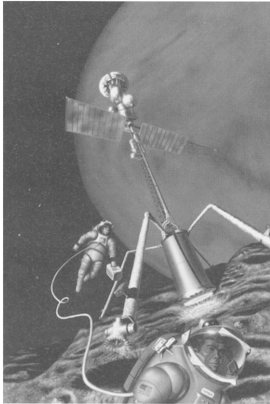
Fig. 12.2 On Phobos, the innermost moon of Mars and likely location for extraterrestrial resources, a mobile propellant-production plant lumbers across the irregular surface. Using a nuclear reactor the large tower melts into the surface, generating steam that is converted into liquid hydrogen and liquid oxygen. (Artwork by Pat Rawlings of Eagle Engineering. S86-25375, 1986. Courtesy NASA) See Plate 17 in color section.
