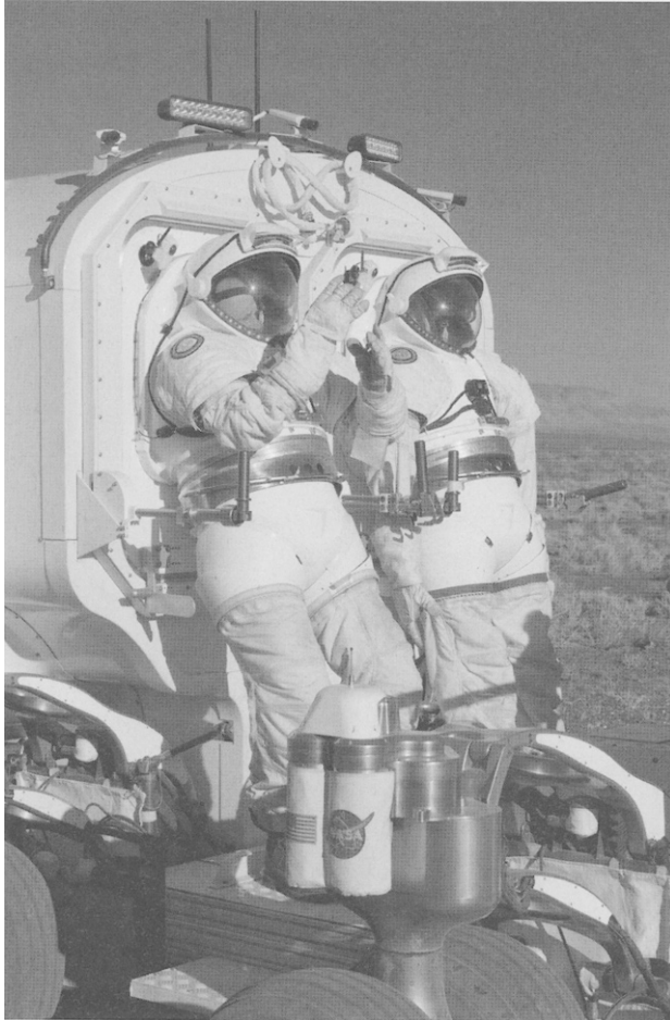
Fig. 8.2 During tests conducted for NASA's Desert Research and Technology Studies (RATS) at Black Point Lava Flow in Arizona, engineers, geologists and astronauts gathered to test two configurations of NASA's newest lunar rover prototype. The pressurized version, seen here and called the Lunar Electric Rover, includes a suitport that would allow crew members to climb in and out of spacesuits quickly for moonwalks. Here, Smithsonian Institution geologist Brent Garry dons his suit. (JSC2008-E-139049, 18-31 October 2008. Courtesy NASA)
