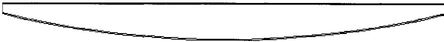
Fig. 6.13 The shape of the floor tie. This shape was chosen to match the bending moment in the tie, thicker where the moment is largest. (Courtesy Florian Rues)
