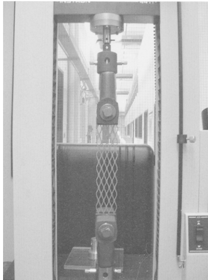
Fig. 9.14 Scale model of intact ribbon under tension.
