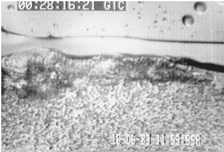
FIGURE 9.13 Video frame showing intermediate phases 4 min after contact in C_{12}E_5 -water- n -tetradecane water system at 45°C near the PIT. (From Benton, W.J. et al., J. Colloid Interface Sci. , 110, 363, 1986. With permission.)
