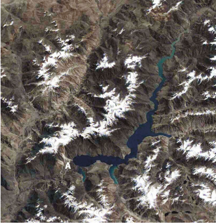
Fig. 1.3 Oblique photograph taken from International Space Station in September 2001 of Lake Sarez, Pamir Mountains, Tajikistan. Lake Sarez is a rockslide-dammed lake impounded by the 1911 Usoi rockslide (A) ([223]; Chap. 7 by Delaney and Evans, this volume). Lake Sarez has a length of ca. 60 km and a volume of ca. 17 Gm 3 (NASA photograph ISS002-E-7524)
