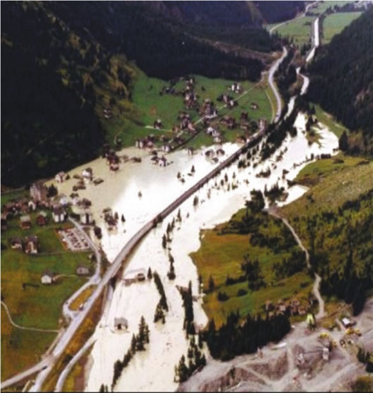
Fig. 3.12 Due to a debris flow which blocked the provisional excavation channel, the plain below the village of Randa was flooded for a short while. The road was maintained by a floating bridge set up by the Swiss army (photograph supplied by CREALP)
