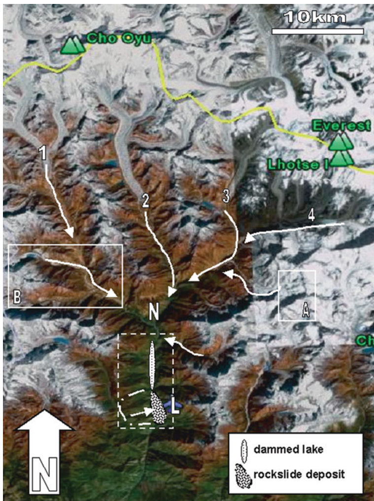
Fig. 8.19 Overview of the catchment area of Gath-Chaunrikharka rockslide dam (source: Google Earth): 1 – Nangpa glacier, 2 – Ngozumpa glacier, 3 – Khumbu glacier, 4 – Lhotse glacier. L – Rockslide deposit close to Lukla, scarp and formerly dammed lake (shown in Fig. 8.18), N – Namche Bazar village; inferred tracks of prehistoric and recent GLOFs in the Khumbu area (white arrows), which may have been contributed to infilling of the former dammed lake: A = Nare Dranga from Ama Dablang South Glacier (6,856 m a.s.l), which occurred in 1977, B = Dig Tsho from Langmoche glacier, which occurred in 1985, and other possible sources in upper tributary valleys (after [53])
