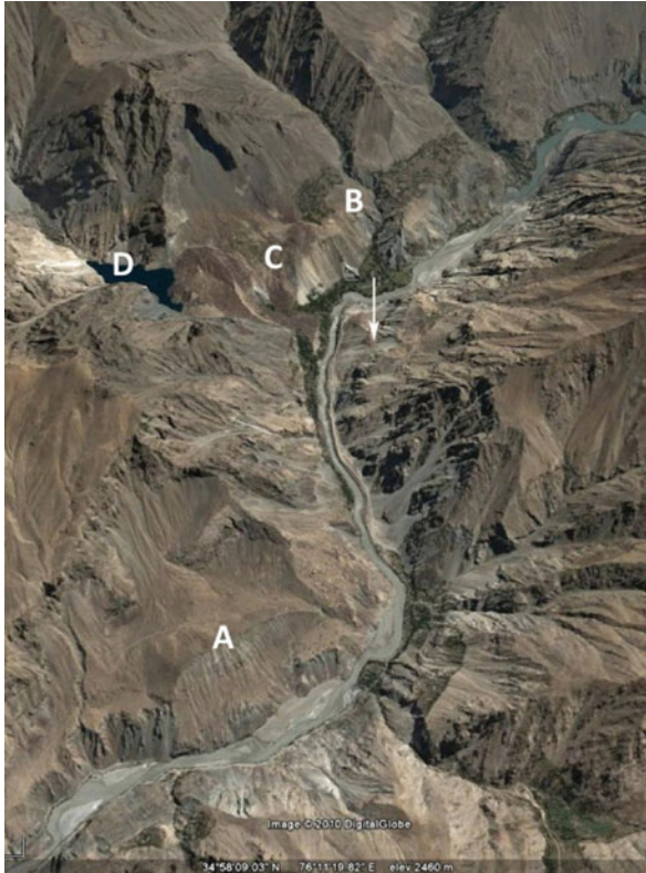
Fig. 7.5 Typical example of complex valley fill deposits in the Upper Indus basin, northern Pakistan. Previously unmapped deposits include (1) older rockslide deposits at A and B that both dammed the Indus River, (2) younger rockslide deposits (C) that have dammed a tributary forming a rockslide-dammed lake at D and ran up the opposite valley slide to a limit indicated by vertical arrow . This rockslide also dammed the Indus. Length of Indus (flowing from top right to bottom left ) seen in image is 13 km. Google Earth image at 34^{\circ} 58' 09''\text{N}/76^{\circ} 11' 19''\text{E} , 65 km SW of Skardu. Locality is indicated in Fig. 7.3
