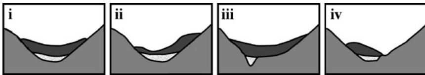
Fig. 24.6 Four types (i–iv) of cross valley profiles of rockslide deposits and underlying valley morphologies
