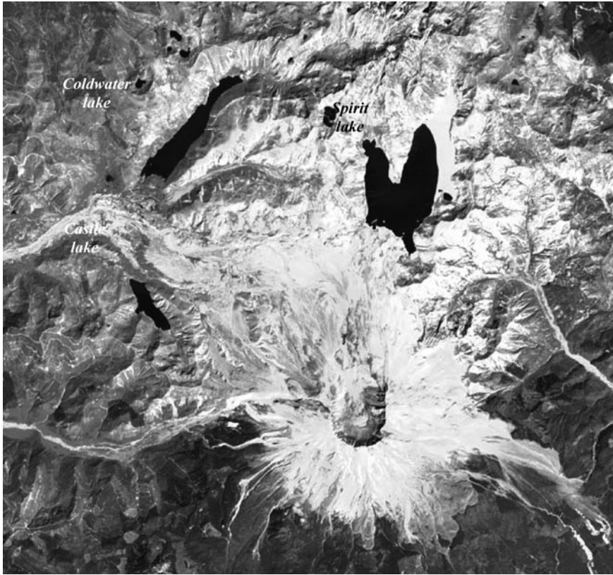
Fig. 9.1 ASTER image of Mount St. Helens showing the two new lakes (Coldwater and Castle) formed by the emplacement of the debris avalanche deposit during the May 18, 1980, eruption. The pre-existing Spirit Lake underwent an increase in water level of approximately 60 m
