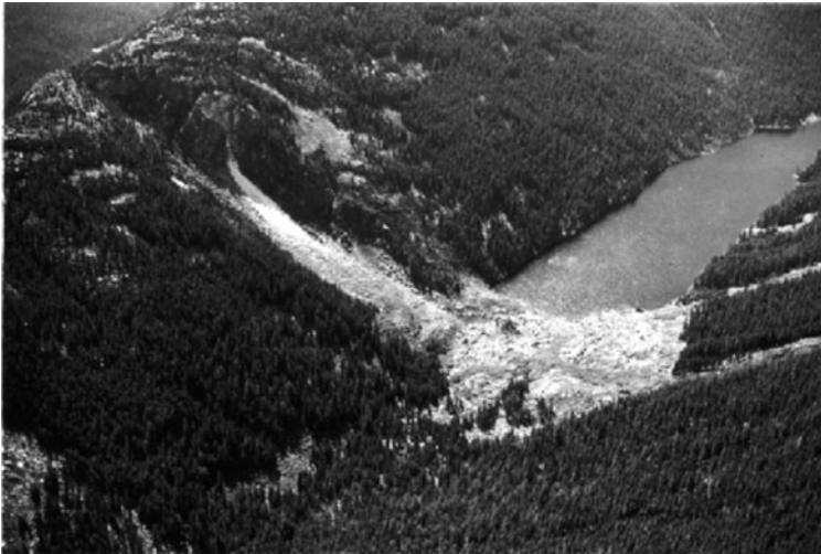
Fig. 1.6 Rockslide-dammed lake in the Coast Mountains of British Columbia formed where a rock avalanche of unknown age has blocked the Nahatlatch River ( 49^{\circ} 53' 32'' N/ 121^{\circ} 50' 19'' W)
