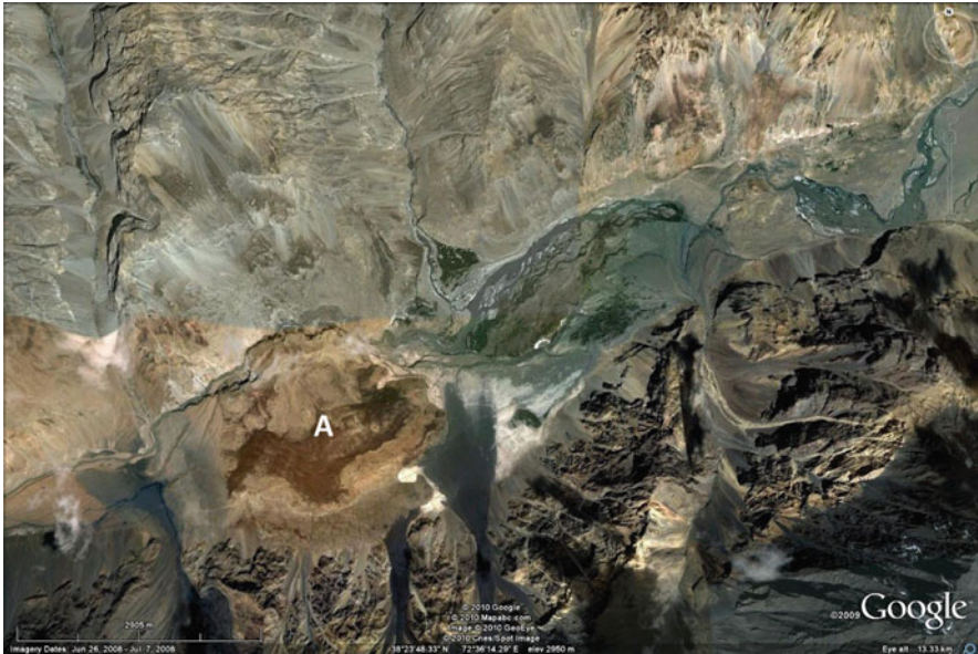
Fig. 7.16 Google Earth image of the gigantic Pasor rockslide (A) that has blocked the Bartang River (flowing from right to left ) in the Pamirs of Tajikistan at 38^{\circ} 23' 03''\text{N}/72^{\circ} 34' 49''\text{E} . The rockslide debris extends 2.72 km across the valley floor and has a volume in excess of 500 \text{ Mm}^3
