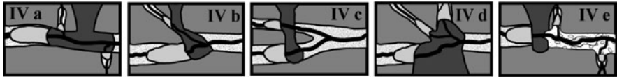
Fig. 24.4 Five sub-types (IVa–e) of plan view distribution of single rockslide dams forming two or more dams in a single valley in a line
