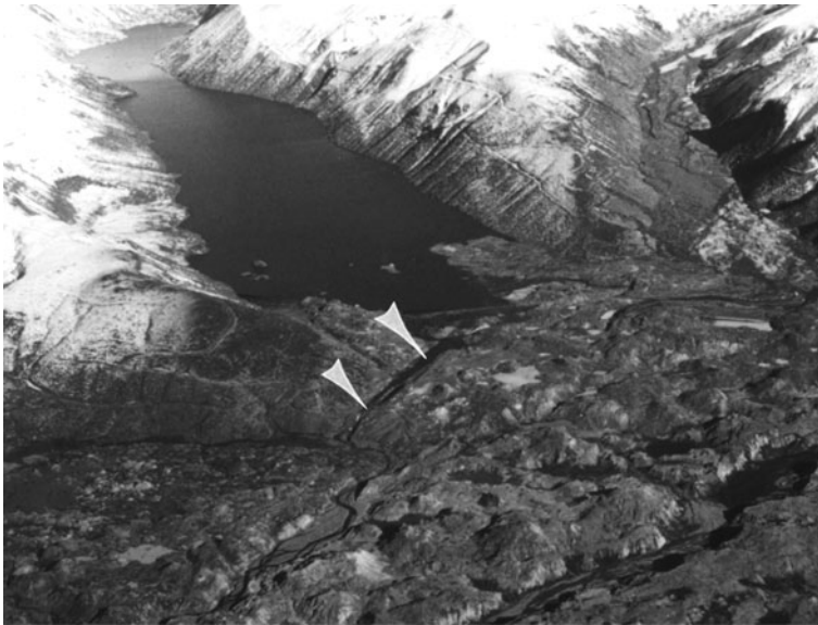
Fig. 2.8 Coldwater Lake and the debris-avalanche blockage of Coldwater Creek, near Mount St. Helens. Location of the excavated channel spillway across the right volcanic-bedrock abutment is indicated by the white arrows
