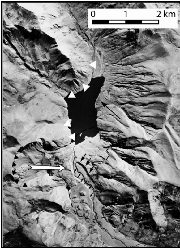
Fig. 5.13 Air photo with interpretation of Navarrete Lake and partially eroded rock avalanche dam ( dashed line ) after [31, 41, 42]. It is interpreted that the dam breached in a catastrophic event as indicated by the steep walled canyon eroded into the crown of the rock avalanche deposit ( large black arrows ) and the inundation surface spanning the entire width of the valley surrounding highest hummocks of the rock-avalanche deposit downriver the canyon, which in turn is cut by a steep walled gorge ( small arrows ). A palaeoshoreline surrounding the lake at a relative elevation of 40 m ( white triangles ) indicates that the lake level was stable for a long time before dam failure. A possible reason for failure is landsliding into the lake by a massive debris flow from the E-side of the lake ( large black arrow ), generating a displacement wave overtopping the dam crown and causing intensive erosion of the dam. This debris flow deposit appears to be young and does not show the palaeoshoreline; hence it was deposited simultaneously with or subsequently to dam failure
