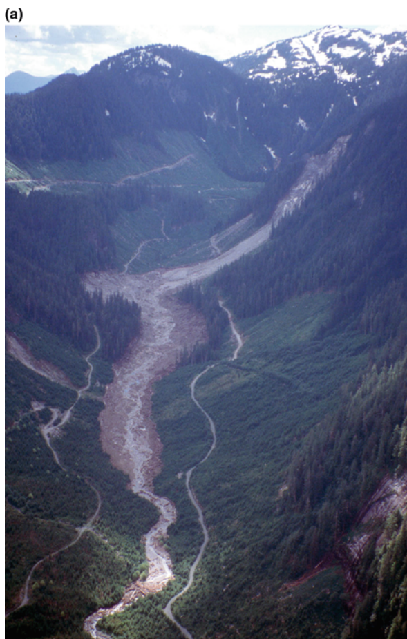
Fig. 18.11 Analyses of the Nomash River rock slide debris avalanche using the program Dan3D [17]. (a) An aerial view of the slide. (b) Analysis using the Voellmy fluid model as described by Hungr and Evans [10]. (c) Analysis using the frictional model, with a bulk friction angle of 20^\circ . The depth contour interval is 2 m. The thin line is the actual path outline. Time intervals 25 s
