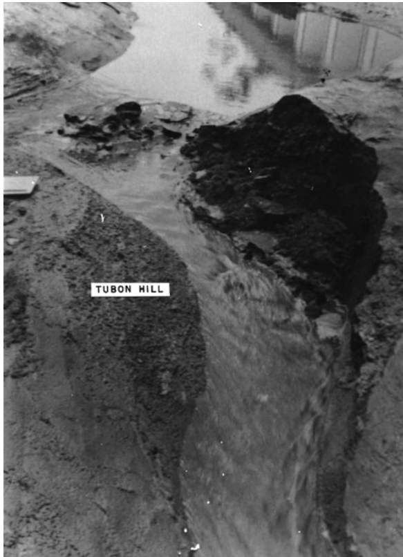
Fig. 14.9 Erosion in the physical scale model, view upstream, tested by EPN technical team [28]
