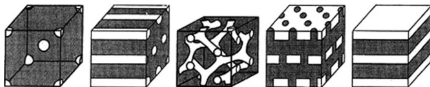
Fig. 1 Schematic representations of the morphologies obtained for diblock copolymer melts. Reprinted with permission from Khandpur et al. [12]. Copyright 1995 American Chemical Society
