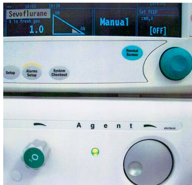
FIGURE 38-19. Enlarged view of concentration dial and agent display box on screen. Although this is an electronically controlled vaporizing system, agent concentration is increased by turning the dial in a counterclockwise direction, analogous to the dial on a traditional variable-bypass vaporizer (e.g. Tec 7, Dräger Vapor 2000.)
