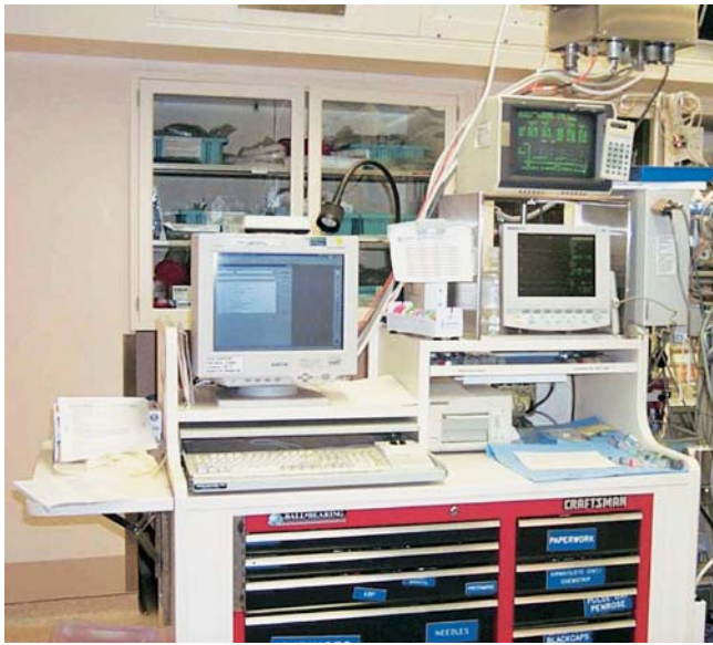
FIGURE 28-8. Anesthesia cart in the cardiovascular operating room. Physiologic monitor and anesthetic gas analyzer on right. Computer screen and keyboard on left. Computer itself is mounted on the back of the cart.
