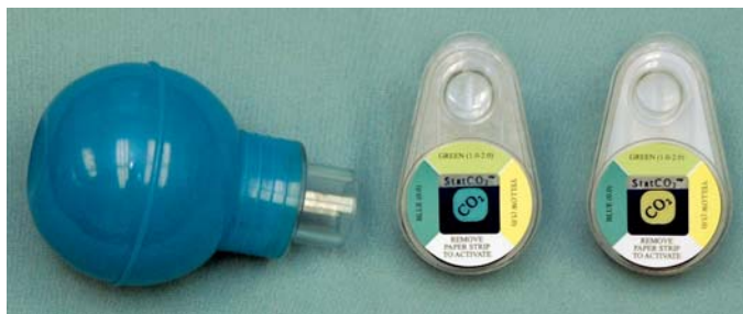
FIGURE 35-32. Self-inflating bulb fitted with a standard 15-mm adapter used as an esophageal detector device. Disposable CO 2 detector showing the green color change to yellow color with CO 2 exposure.
