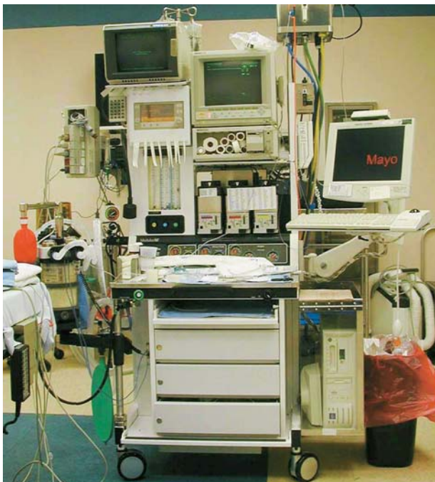
FIGURE 28-9. Mounting of the PIMS hardware in general purpose operating room. Flat screen monitor and keyboard mounted via an articulating arm on right of anesthesia machine. Computer is below on a custom shelf affixed to right side of the machine.
