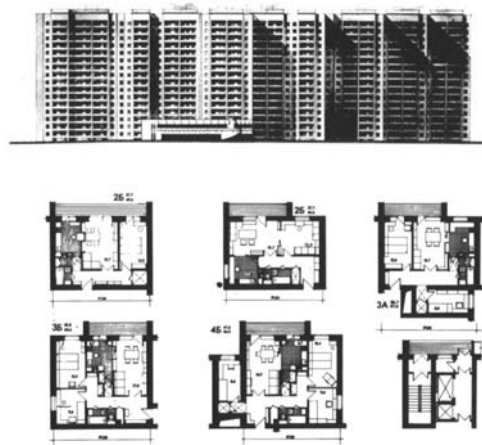
Figure 5.16 Systematic design series K-134 for the new residential district in Kiev. (Department of Systematic Designs of the State Design Institute for Civil & Industrial Construction, Kiev, Ukraine.)
