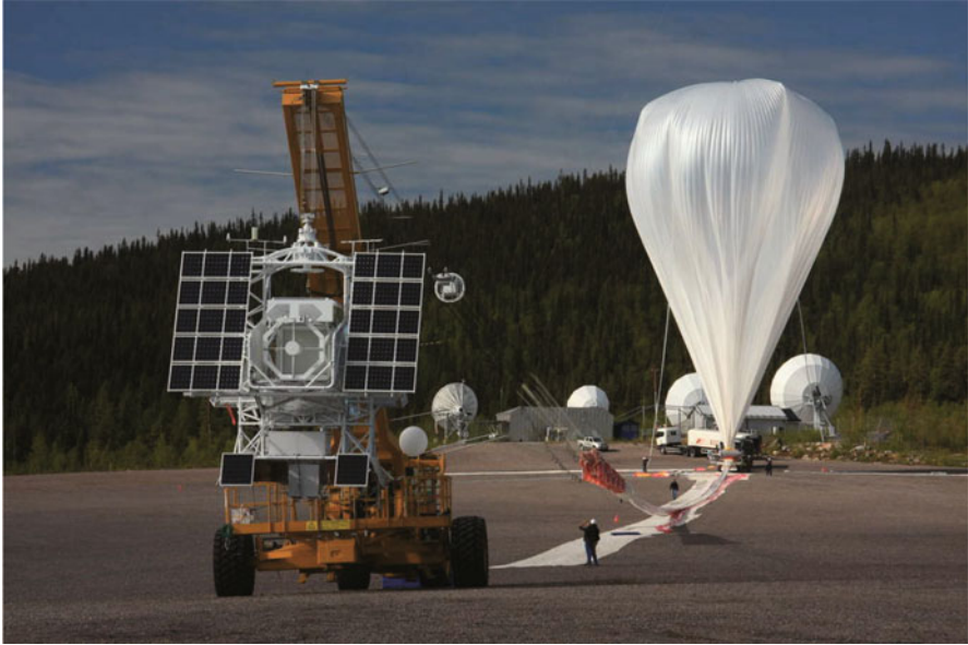
Fig. 21.3 SUNRISE balloon-borne stratospheric telescope. The 1 m aperture telescope is mounted on a gondola
