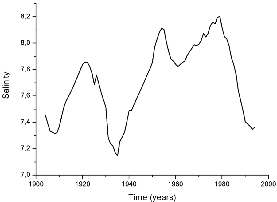
Figure 2.16. Annually, horizontally, and vertically averaged Baltic Sea mean salinity (from Winsor, Rodhe, and Omstedt, 2001, 2003).
