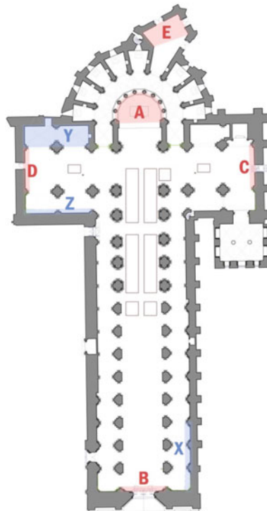
Fig. 6 Location of selected “hot-spots” and “cold-spots”. The projected “hot-spots” were: the apse behind the presbytery (“hot-spot A”), the west façade, with the entrance and the rose window (“hot-spot B”), the south façade (“hot-spot C”), the north façade (“hot-spot D”) and the passage to the Manueline sacristy (“hot-spot E”). The predicted “cold-spots” were: the first three bays on the south wall of the nave (“cold-spot X”) and the east and west walls of the north side of the transept (respectively “cold-spot Y” and “cold-spot Z”)
