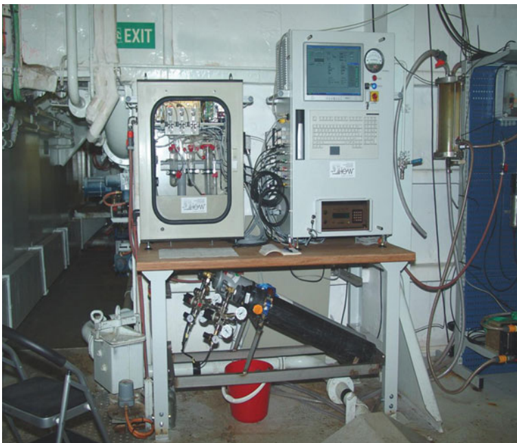
Fig. 3.3 The pCO 2 measurement system on cargo ship FINNMAID. On the table to the left : The ‘wet’ unit where air is circulated in a closed loop through surface water that is pumped continuously into an equilibrator. Right side of the table: The ‘dry’ unit which contains the electronics and an IR spectrometer for the determination of the equilibrium CO 2 concentration (pCO 2 ) of the air circulating through the surface water in the equilibrator
