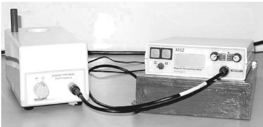
Figure 4.27. MS2 Bartington susceptibility meter attached with a dual frequency MS2B sensor can rapidly measure low field or initial susceptibility. The sensor subjects the sample to a non-saturating field that has the advantage of measuring initial susceptibility without destroying magnetic remanence of the sample.
