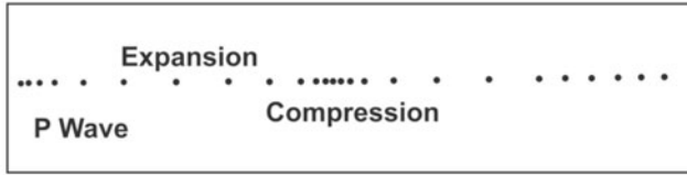
Figure 2.5. The dilatation and compression in the propagation of P wave having longitudinal type particle motion.
