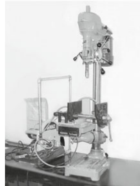
Figure 4.15. Rock coring (right) and rock cutting (left) equipments.
