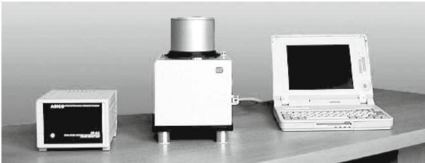
Figure 4.17. Laboratory induced remanent magnetization called anhysteretic remanent magnetization (ARM) and isothermal remanent magnetization (IRM) is imparted and measured by highly sensitive JR-6 spinner magnetometer. Rock and sedimentary samples of defined shape and size rotate at a constant angular speed in the pick-up unit inside a pair of coils. An AC voltage is induced in the coils whose amplitude and phase depend on the magnitude and direction of the magnetic remanence vector of the specimen. By Fourier analysis the computer calculates two rectangular components of the projection of remanence vector into the plane perpendicular to the axis of rotation.
