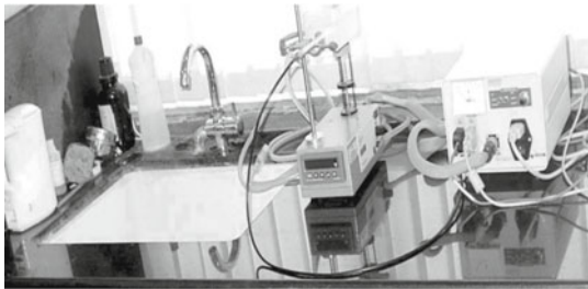
Figure 4.24. Bartington temperature variation of magnetic susceptibility meter, operating over the temperature range -200^{\circ}\text{C} to +900^{\circ}\text{C} , is used to investigate magnetic mineralogy, grain size and for the determination of Curie transition temperatures.
