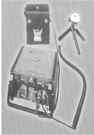
Figure 4.12. Advanced magnetotelluric system that uses 24-bit analog-to-digital converter.
