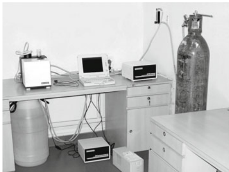
Figure 4.25. Anisotropy of magnetic susceptibility kappabridge (KLY-4S) and temperature variation apparatus (CS-3). The kappabridge is used to measure magnetic susceptibility of rock and sedimentary samples, as also its anisotropy. Its operation is based on measurements of inductivity changes in coil due to a rock/sedimentary specimen. This instrument is attached with high and low temperature apparatus CS-3/CS-L to monitor temperature variations of magnetic susceptibility.
