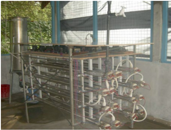
Fig. 4.5 Electrocoagulation plant implemented in rural Sri Lanka (Picture by Mr. J.P. Padmasiri, Institute of Fundamental Studies, Kandy, Sri Lanka)
