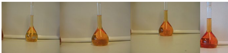
Fig. 5.3 Chemical method for nan-Se synthesis. The ascorbic acid or vitamin C was used plus sodium selenate as a source of Se. It could be distinguished formation stages of the red color of elemental nano-Se. (Photo by H. El-Ramady, Nano Food Lab, Debrecen Uni., Hungary)
