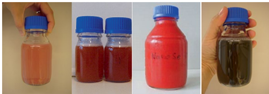
Fig. 5.2 Different possible colors of nano selenium suspension after using of the biological synthesis method, where MRS medium, sodium hydrogen selenite and bacteria strain were used. (Photo by Nano Food Lab, Debrecen Uni., Hungary). For LactoMicroSel we use milk as medium. The milk fat makes further processing hard, as some of the selenium containing bacteria gets attached to the fatty fraction floating at the top, while the others consolidate to the bottom. So we separate the fat from the milk using a separator seen on the top left picture, then we inoculate it with LactoBacteria. We put the inoculated milk into an incubating chamber for 2 days, on 37°. Then, we dry and mill the produced yoghurt. The resulting fine powder is the finished LactoMicroSel product, and its selenium concentration is about 3000 ppm
