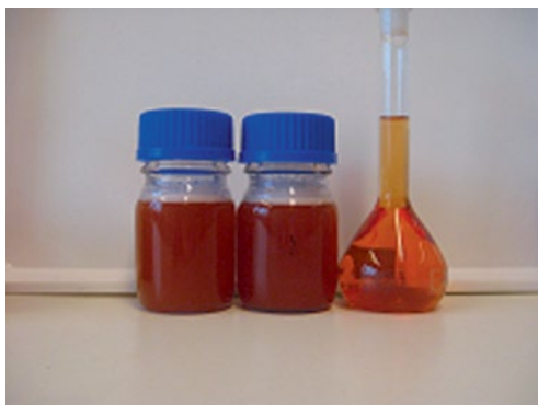
Fig. 5.4 Comparison between biological and chemical methods for nano-Se production. The right 100 measuring flask belongs the chemical method, where it used vitamin C or ascorbic acid and the other flasks are belong to the biological method using MRS media and Lactobacillus casei as a bacteria strain. (Photo by H. El-Ramady, Nano Food Lab, Debrecen Uni., Hungary)
