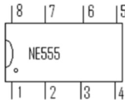
Figure 4-3. The DIP pin numbering scheme
