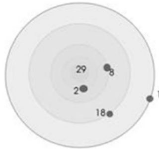
Figure 1-1. The Bohr model of the copper atom
