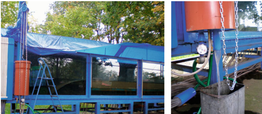
Fig. 1 The flume and the tank that provokes the induced seepage through the sandy layer
