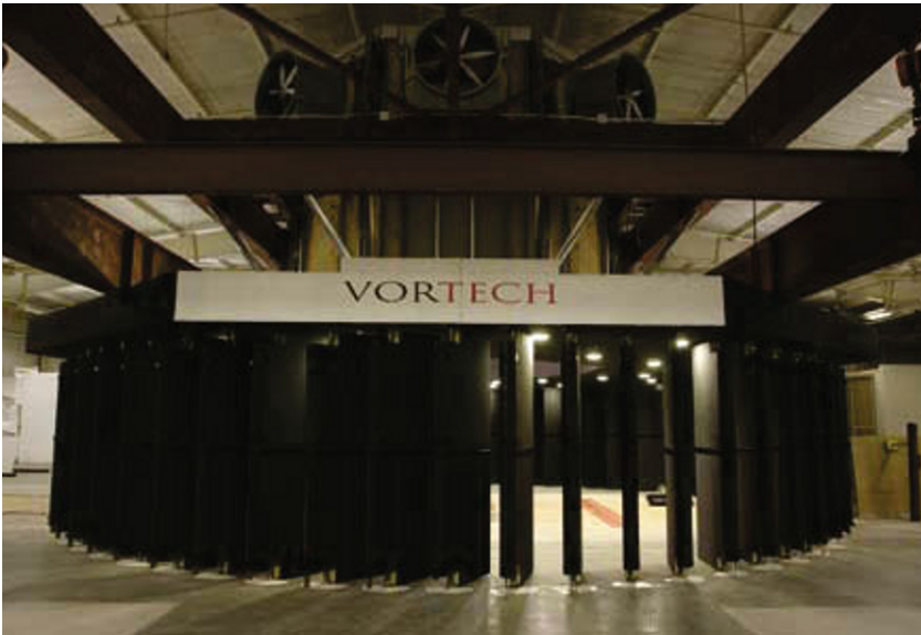
VorTECH: a 10-m-diameter chamber to simulate velocity and pressure profiles of tornado-like vortices at Texas Tech University.
