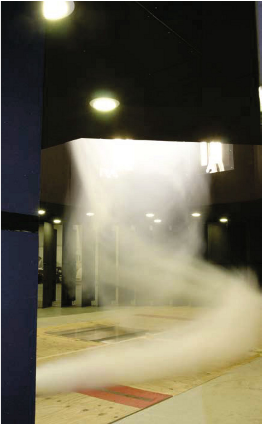
VorTECH tornado vortex simulator at Texas Tech University uses smoke and helium bubbles to simulate the tornado's inner core.
