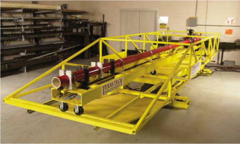
Texas Tech University's Debris Impact Cannon simulates wind-borne debris at 100 mph to test building materials such as doors, windows, and shelters for wind storm safety.
