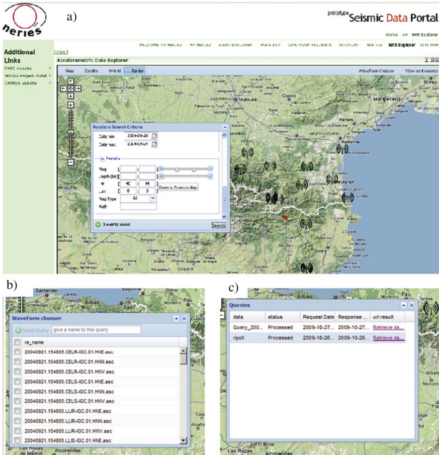
Fig. 9.6 Example of a request to the acceleration data explorer in the seismic data portal with: a the Euro-mediterranean map zoomed in the Pyrenees region, with the epicenters and stations resulting from a query “Accelerometer Search Criteria”; b the list of records available (“Waveform Chooser”); and c status of the download process (“Queries”)
