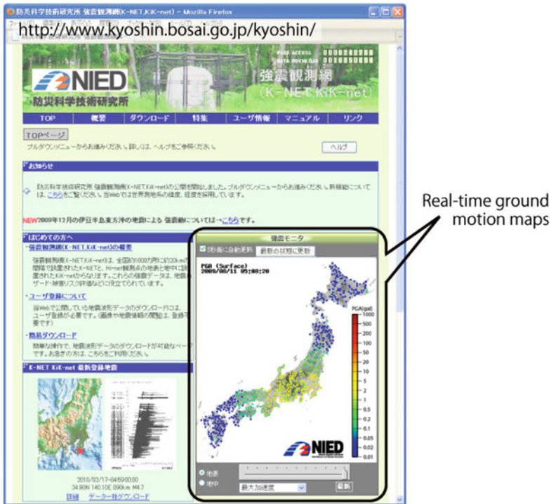
Fig. 12.8 A real-time ground motion map, which is generated from real-time strong motion indexes (PGA, real-time intensity, response spectrum) continuously calculated and telemated from every KiK-net stations every 1 s. The map is routinely shown on web site and automatically re-loaded every 5 s
